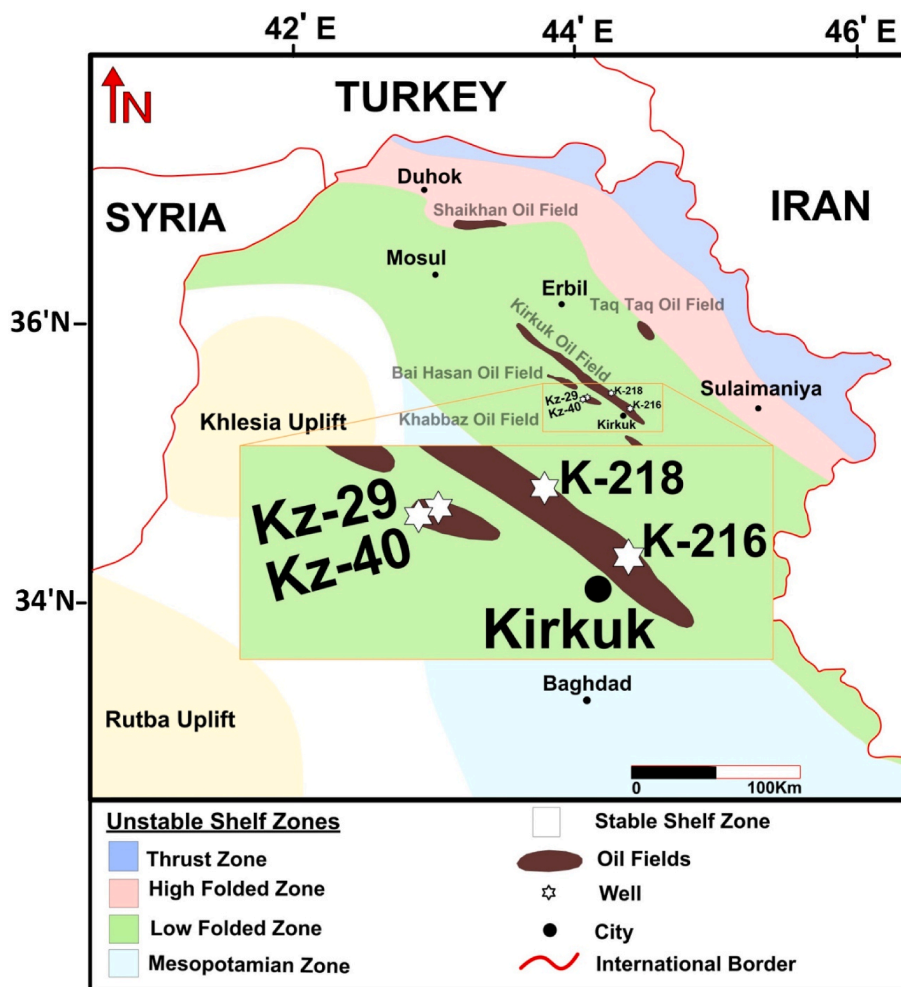
Fig. 1. Map displaying the tectonic divide of Iraq and the locations of the examined wells (Kz-29, Kz-40, K-216, and K-218 wells) [35].
