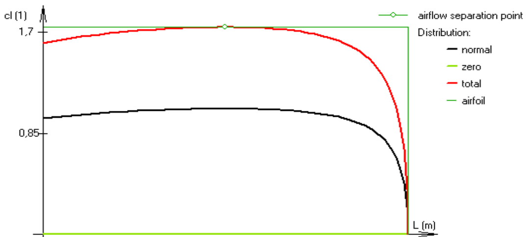
Figure 3.8 Lift distribution along wingspan (Glauert III).
