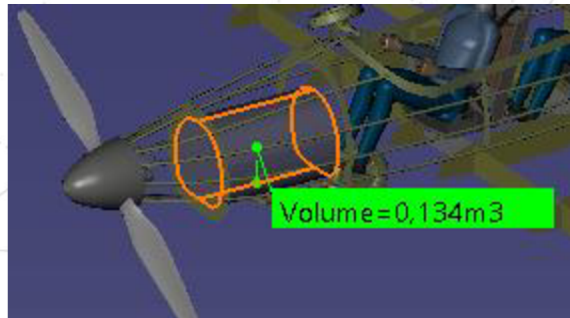
Figure 5.3 Front battery available volume (CATIA).
