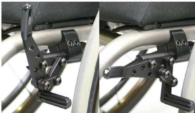
Obr. 9 Brzda push to lock [13].
