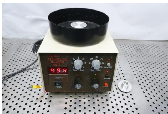
Obr. 18 Spin-coater Chemat technology KW-4A [41].
