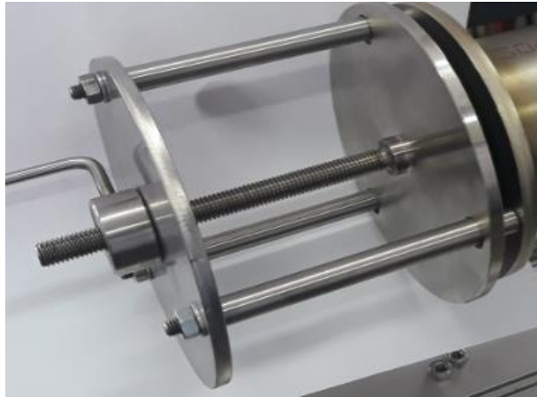
Figure 6.4: Backpressure control assembly.
