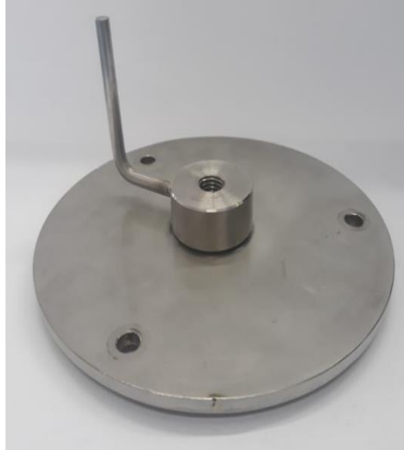
Figure 6.9: Rigid plate welded with ring and handle
