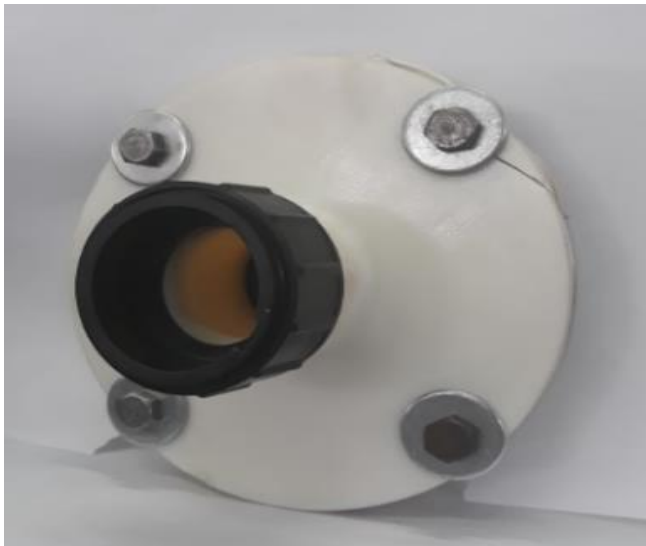
Figure 6.2: Fan Inlet Section.
