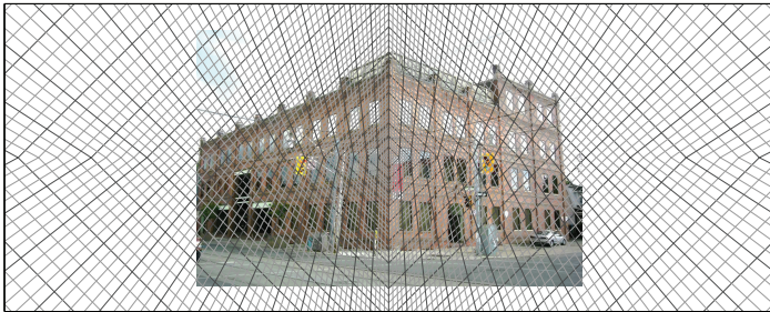
Figure 13: Visualization of the accumulator bins from the diamond space back-projected to the image plane.
