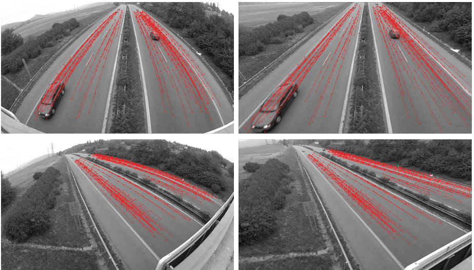
Figure 29: Examples of real-life videos: Radial distortion estimation and compensation.
