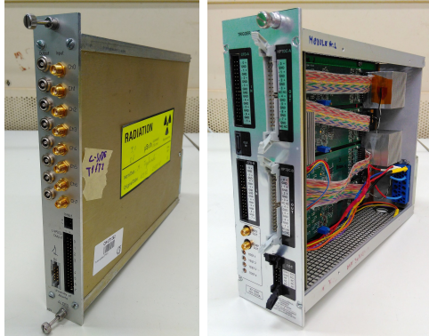
Figure 6.18: The CFD module ( left ) and the trigger module ( right ).
