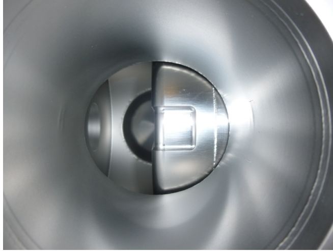
Figure 1.15: View of the Roman pot inserted in the beam pipe [12].
