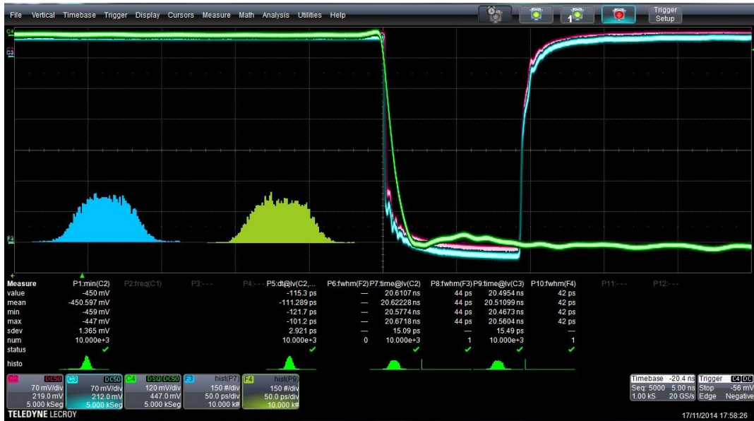
Figure 7.6: Oscilloscope screenshot from the CFD test. Two CFD output channels (magenta and cyan) and the trigger pulse (green) are recorded. The two histograms show time difference between the leading edge of the CFD output w.r.t. the trigger pulse leading edge (at 50% level).
