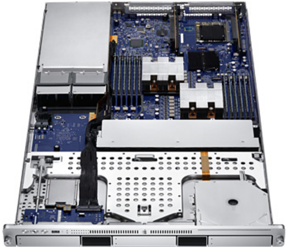
Picture 6-5 Inside of Apple XSERVE "XEON", rack photo
