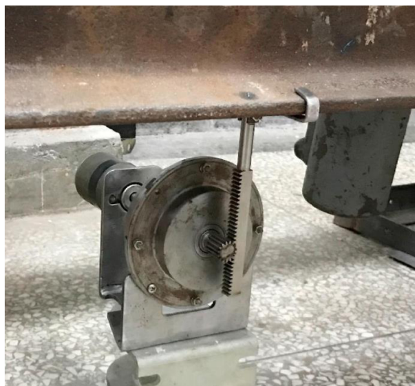
Obr. 11 Jednoduchý MMR energy harvester [17]
