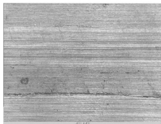
Fig. 16 – Example of abrasive wear from hard sharp particles trapped between moving surfaces [22]
