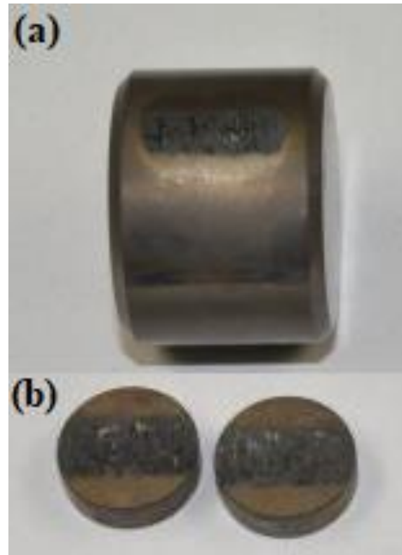
Fig. 56 - Specimens, pin (a) and plates (b) after experiment on DN55 Tribometer
