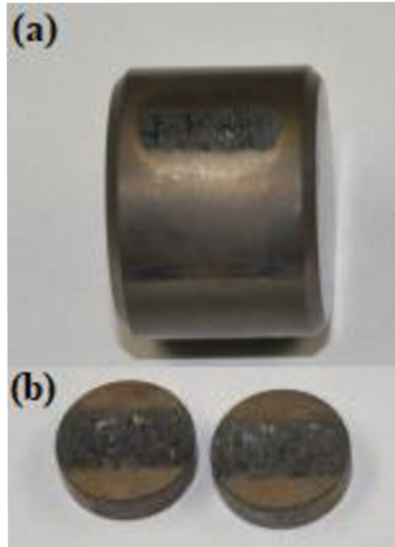
Fig. 56 - Specimens, pin (a) and plates (b) after experiment on DN55 Tribometer
