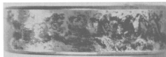
Fig. 20 – Example of fretting wear from the small oscillatory movements between two smooth surfaces [22]
