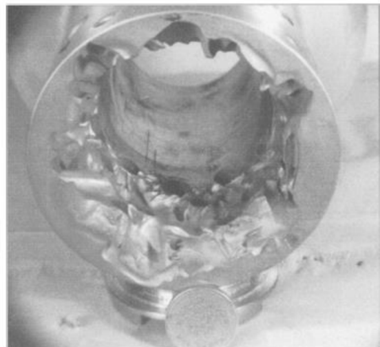
Fig. 24 – Example of particle erosion from hard particles in a stream of fluid [22]
