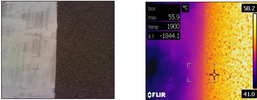
Figure 59. Visible and infrared image of white Paint on Asphalt Surfaces (19 June 2022, at 13.52).
