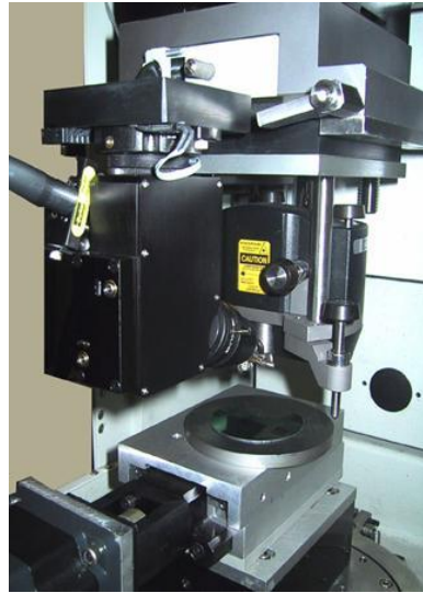
Fig. 4.8: UMT Multi-Specimen Test System used for the analyzing scratch resistance of the composite samples
