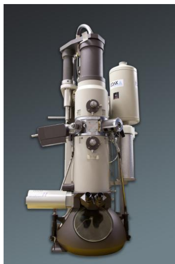
Fig. 5.6: JEOL JSM-2010 Transmission electron microscope
