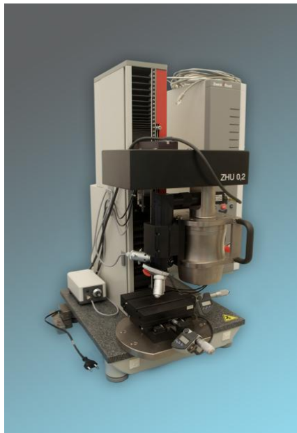
Fig. 4.5: Computer-controlled micro-hardness tester (Zwick/Roell ZHU/Z2.5)
