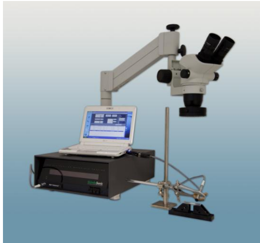
Fig. 4.4: GrindoSonic Mk5i setup for the measurement of the Young's modulus of bar samples
