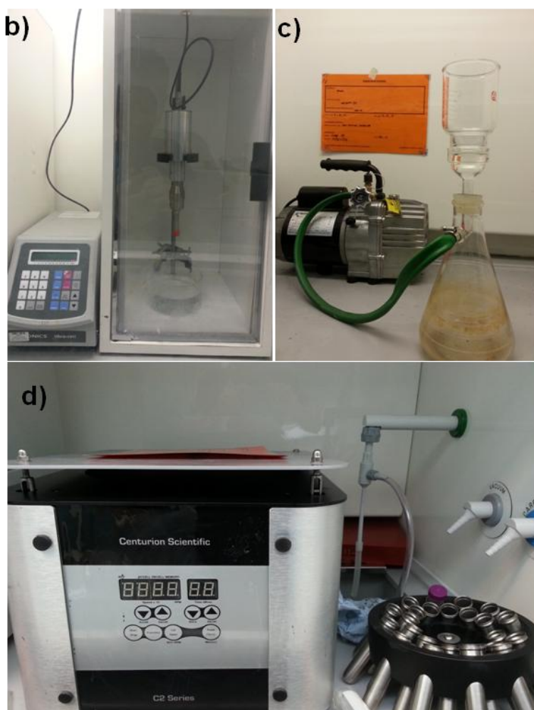
Fig. 5.2: Liquid phase exfoliation of BNNs; a) schematics of exfoliation of BNNs; b) Ultrasonication probe; c) Filtration unit; d) Centrifugation setup
