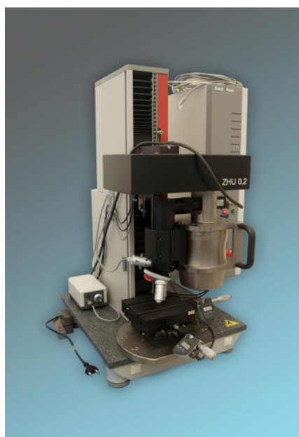
Fig. 4.5: Computer-controlled micro-hardness tester (Zwick/Roell ZHU/Z2.5)
