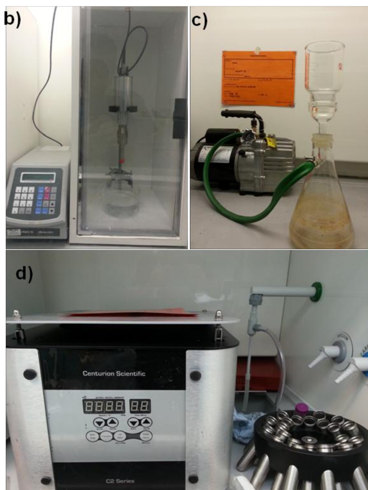
Fig. 5.2: Liquid phase exfoliation of BNNSs; a) schematics of exfoliation of BNNSs; b) Ultrasonication probe; c) Filtration unit; d) Centrifugation setup
