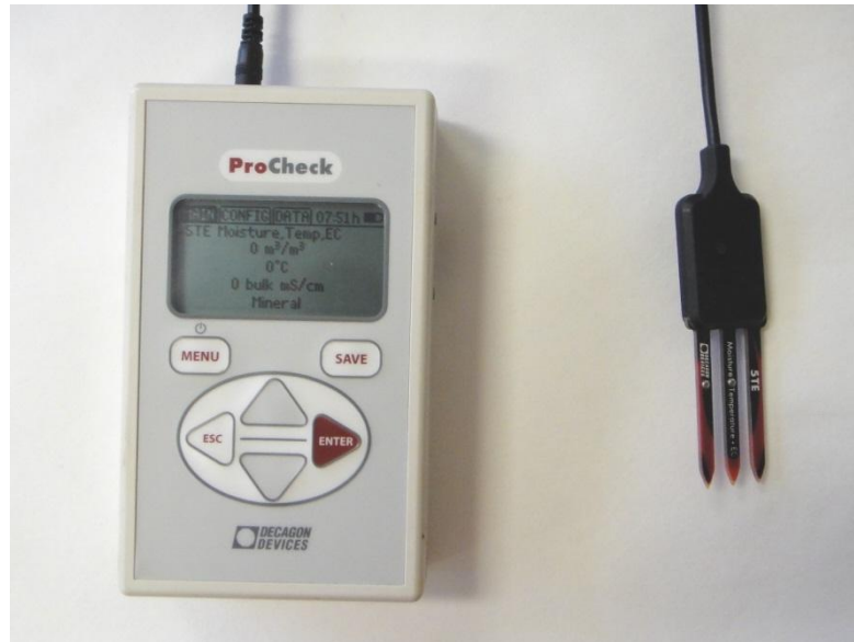
Figure 16 Photo of FDR soil moisture sensor: 5TE Soil Moisture, Temperature, and Electrical Conductivity (Decagon Devices, Inc.)
