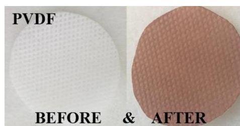
Figure 3.3 PVDF membrane before and after first step surface modification
