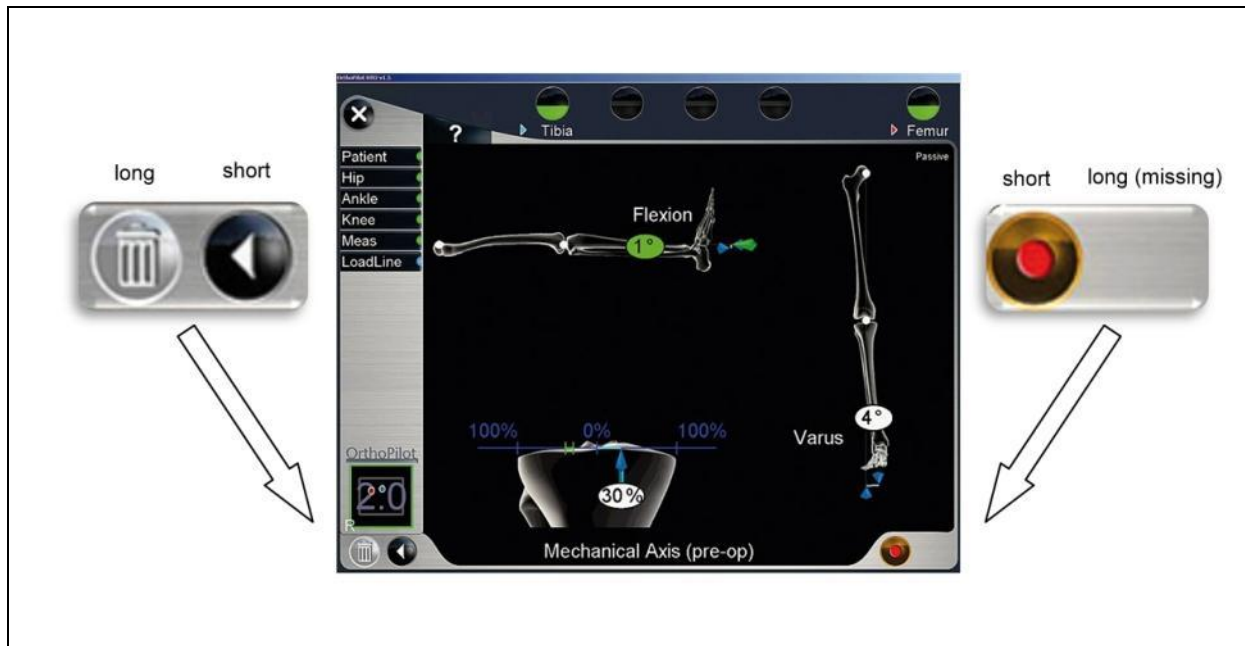
Figure 8: OrthoPilot HTO v 1.5 - different button events. Notice that right long action (moving step forward) as well as left long action (erasing collected data ) is not available as the data were not collected yet. It is done by pressing right button.
