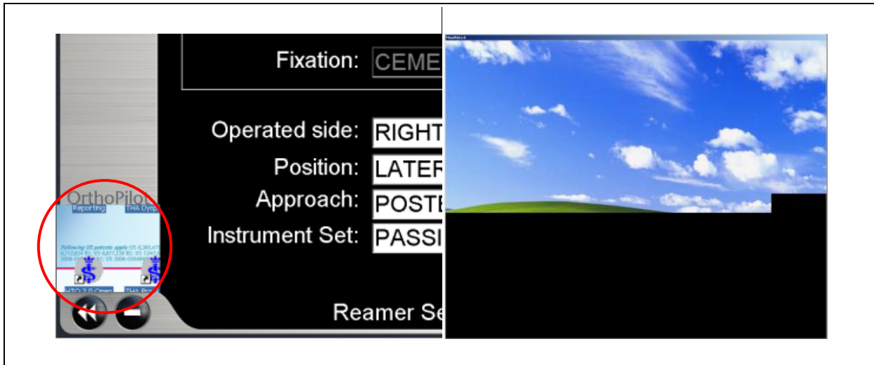
Figure 28: MaxiVista software: left: detail showing problem in TKA application with displaying certain components (hardware acceleration), right: flickering/loading the screen when the program starts
