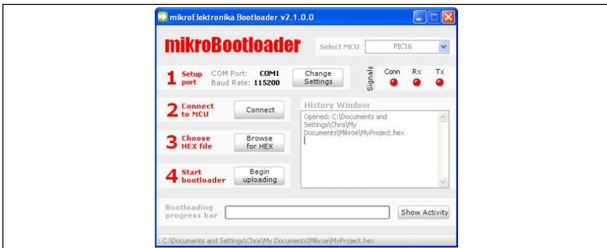
Figure 70: microBootloader software for loading created source code (compiled in HEX code) into microcontroller's flash memory
