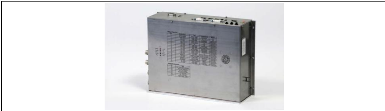
Figure 10: PENTA embedded PC unit
