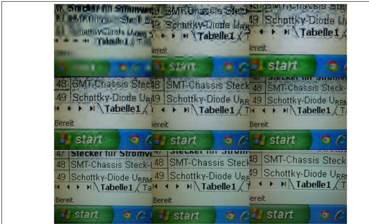
Figure 31: Quality of image depending on bit rate (from left top): 10, 30, 50, 70, 90, 10,130, 150 Mbps, original
