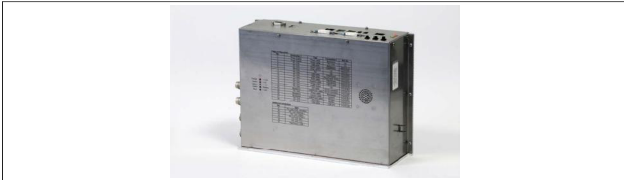
Figure 10: PENTA embedded PC unit
