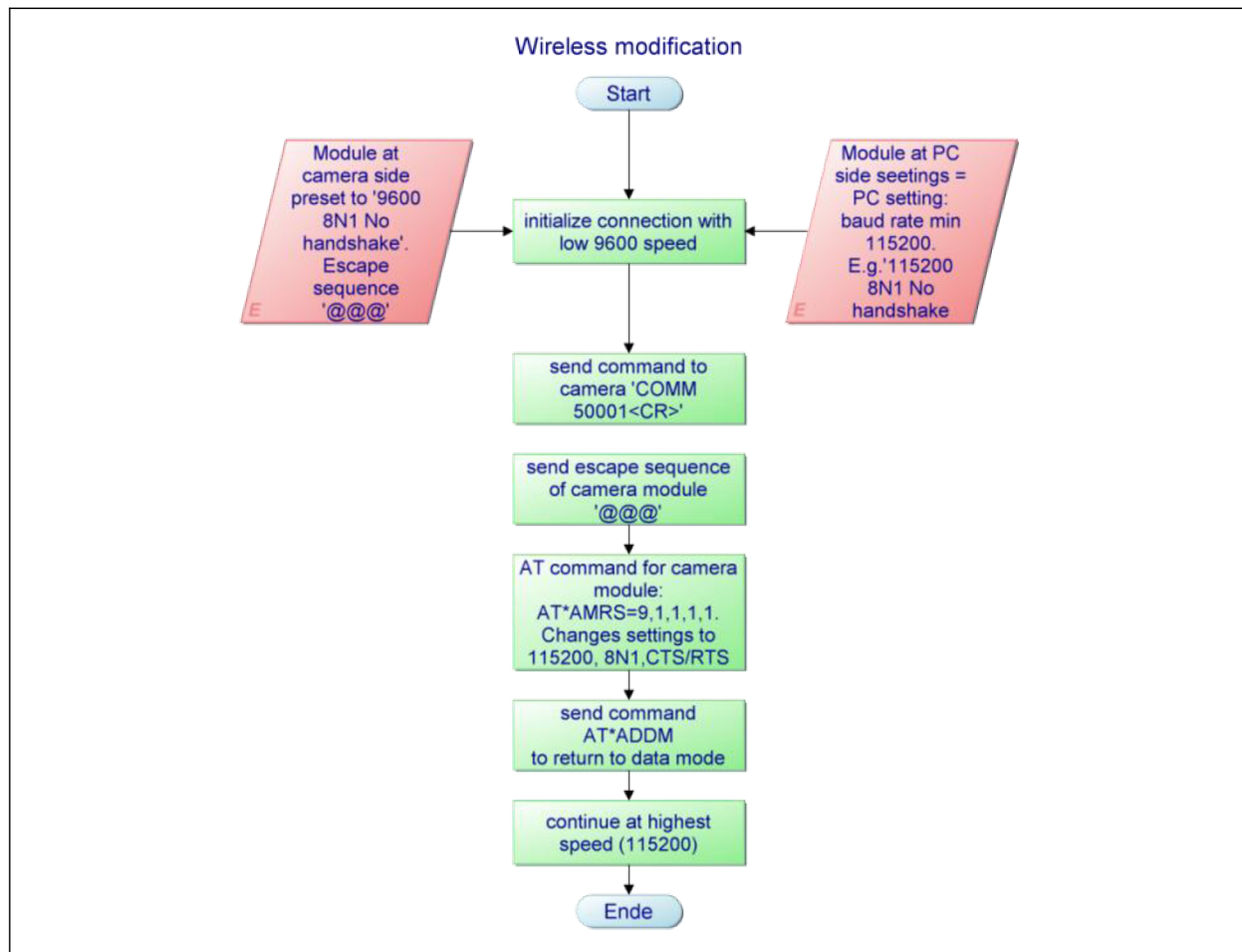
Figure 65: Camera initialization wireless module modification
