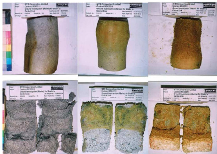
Figure 2.3 Triaxial Specimen of Alluvium
