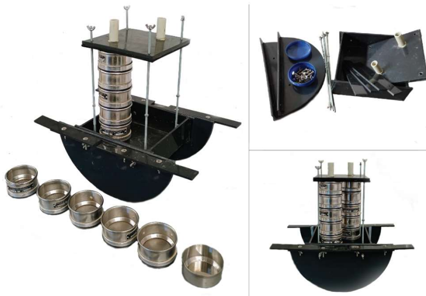
Figure 16: Manual tilting device for possibility to work in the field. Visualised by author.
