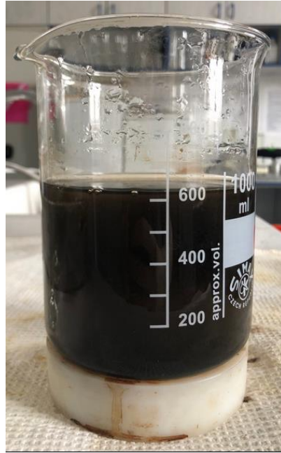
Figure 18. Microwave synthesized magnetite on the NdFeB magnet (author's archive)
