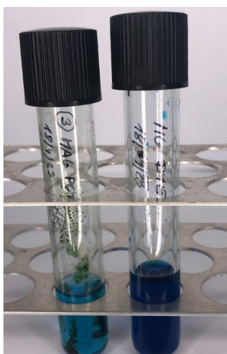
Figure 29. Difference between the sample of dye (5 ml 0.1 mg/mL) with 1000 \mu\text{L} magnetized Pcy and 5 mL of 0.1 mg/mL MG after 24 hours of incubation at laboratory temperature (author's archive)
