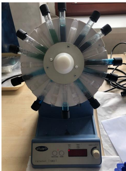
Figure 20. Solution of magnetised picocyanobacteria and dye left for the incubation on the rotator (author's archive)
