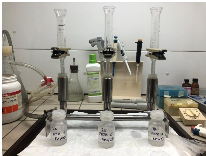
Figure 13. The apparatus used for the purpose of DAPI staining of picocyanobacterial cells and counting filter preparation (author's archive)
