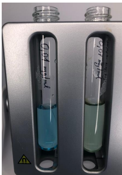
Figure 30. Colour difference in the sample with 500 \mu\text{L} MW Mag Pcy with 5 mL of 0.1 mg/mL MG dye (on the left - dye without the MW Mag Pcy; on the right dye with MW Mag Pcy after 24 hours of incubation) (author's archive)
