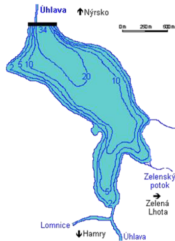
Figure 6. Scheme of the water reservoir Nýrsko (depths in the individual sections marked) (Retour, 1998)
