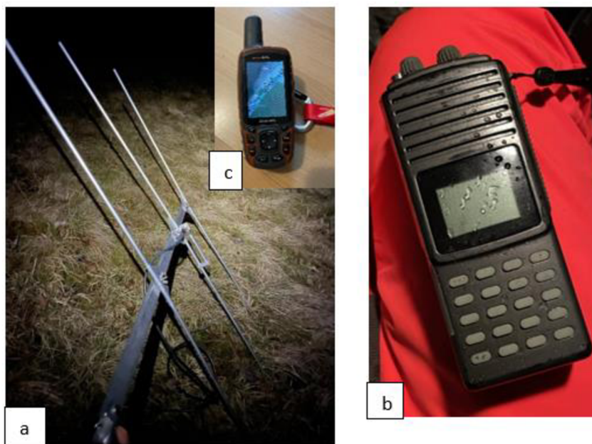
Figure 12: a) antenna, b) receiver and c) GPS Garmin system used for telemetry.
