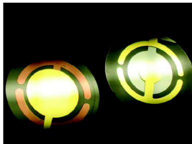
Fig. 4 Quartz crystal microbalance [20]
