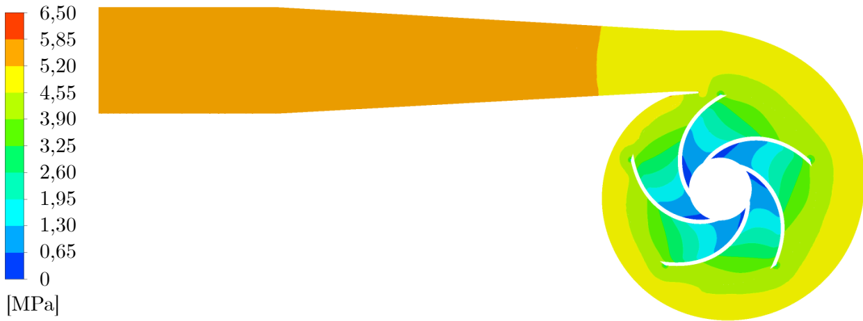
Fig. 1.60: Distribution of static pressure in mid plane for eccentric rotor for f_{\Omega} = 0,5
