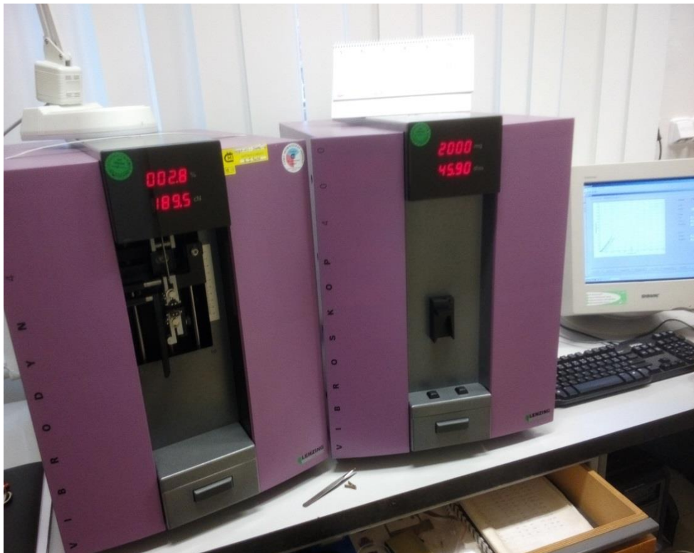
Figure 21. Vibrodyne equipment used for tensile properties of Jute fiber.
