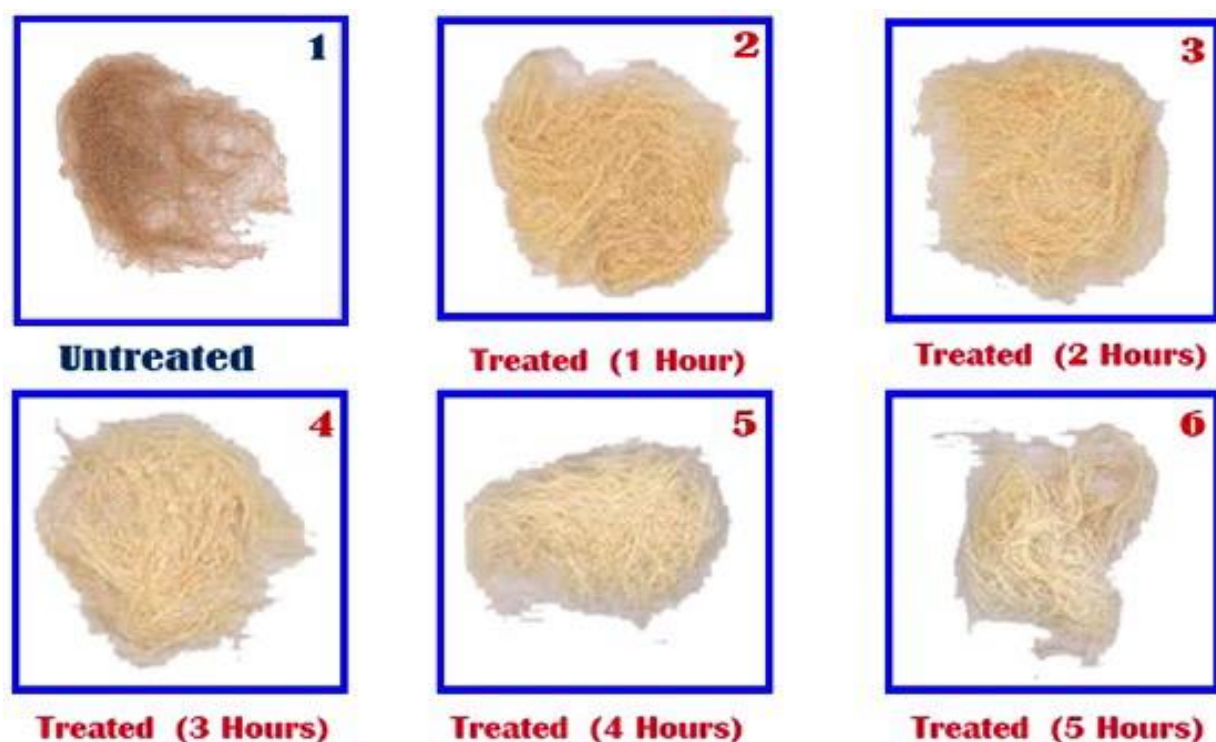
Figure 18. Apparent change in color of untreated and Ozone treated samples of jute
