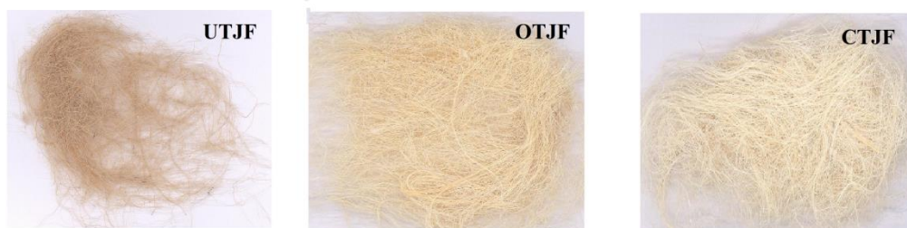
Figure 30. Change in color of jute fibers after pre-treatments
