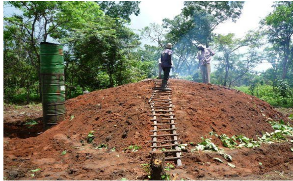
1. Casamance kiln with chimney made of oil drums
