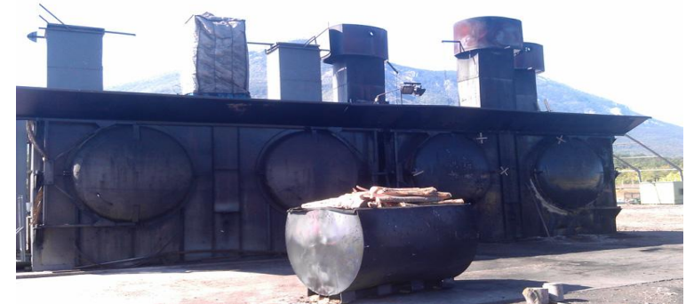
4. Modern furnace for charcoal production with Van Marion system
