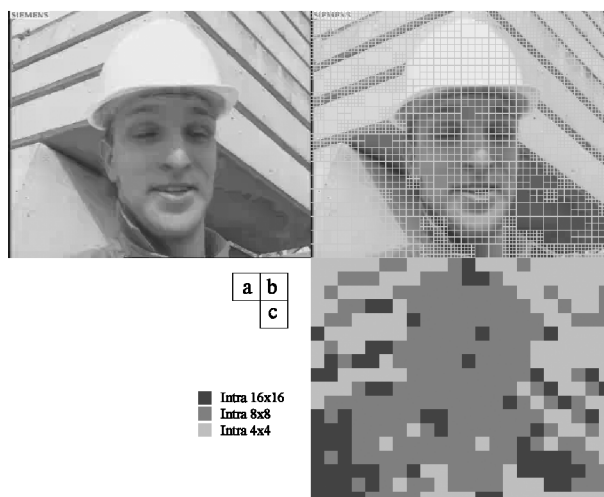
Figure 3.10: Foreman sequence, frame 0, PSNR = 33.83 dB, QP = 35.
