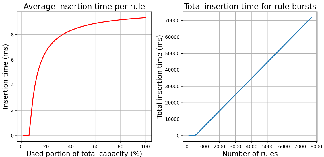
Figure 6.3: Average and total insertion times for rule bursts on NICs with I40E PMD.
