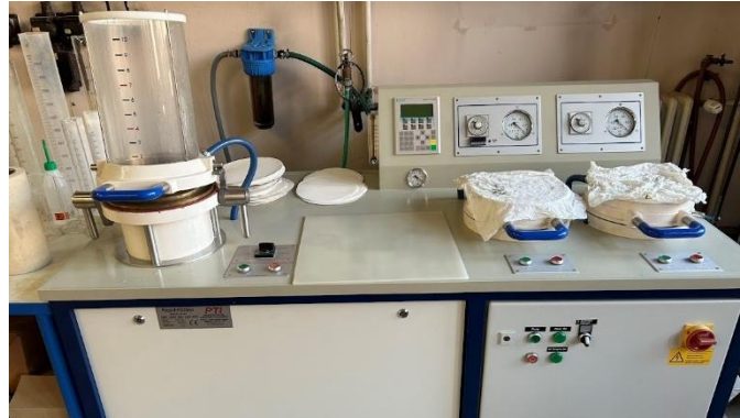
Figure 22: Standardised hand sheet production machine
