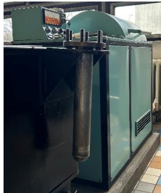
Figure 18: Hot oil pulp cooker VŠ-01/84
