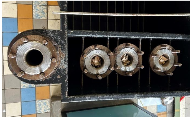
Figure 17: Cooking pressure vessels, Hagglung bombs
