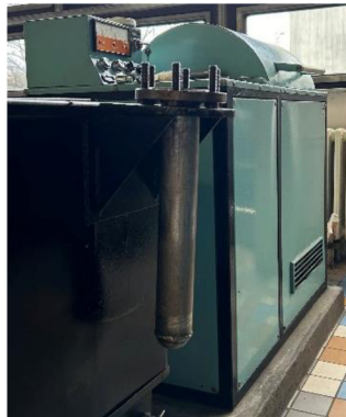
Figure 18: Hot oil pulp cooker VŠ-01/84
