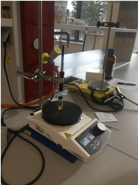
Figure 15 Exposed fiber in the headspace of the vial
