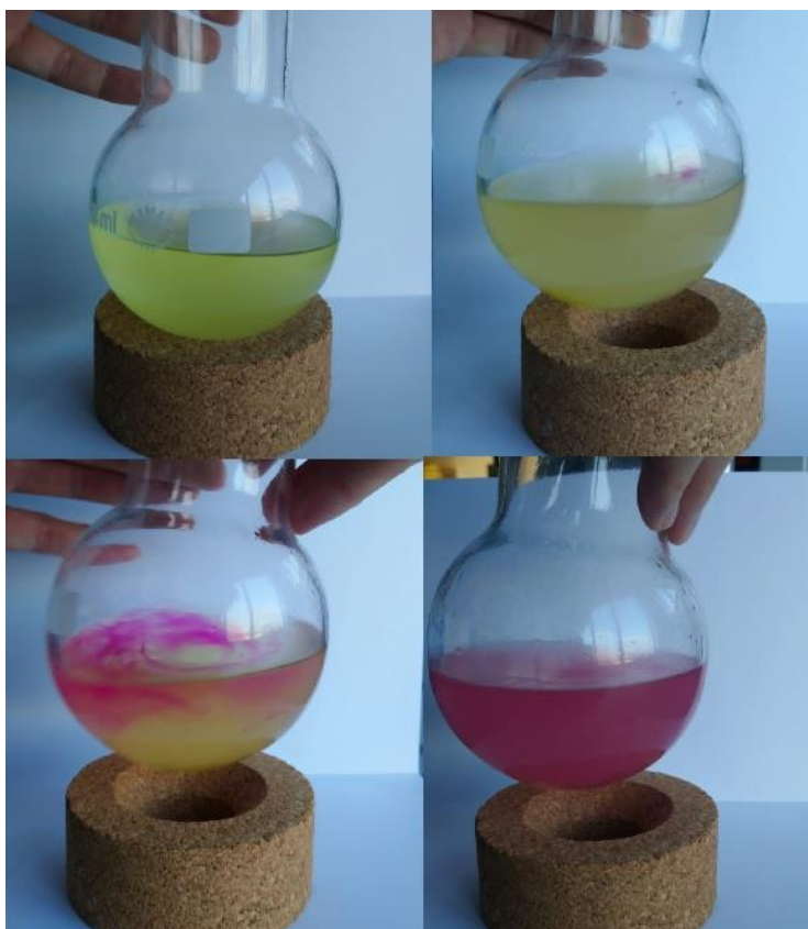
Figure 14 Acid value sample during titration
