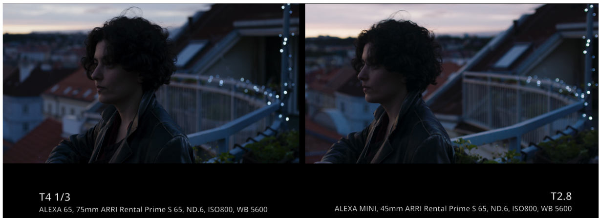
Still 8 - Matching depth of fields by closing the aperture on the Alexa 65
