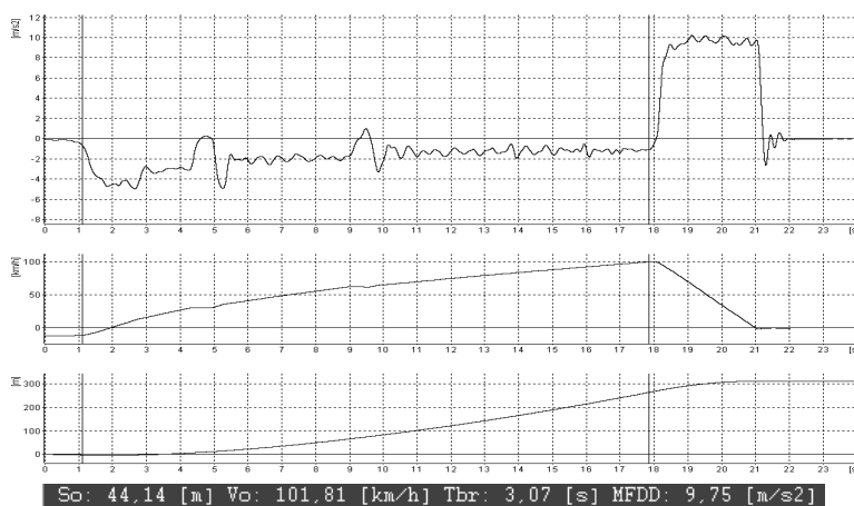
Fig. 5. Peugeot 301, v_0 = 101,81 \text{ km}\cdot\text{h}^{-1} , temperature 22 \text{ }^\circ\text{C} , GoodYear GT3 Obr. 5. Peugeot 301, v_0 = 101,81 \text{ km}\cdot\text{h}^{-1} , teplota 22 \text{ }^\circ\text{C} , GoodYear GT3
