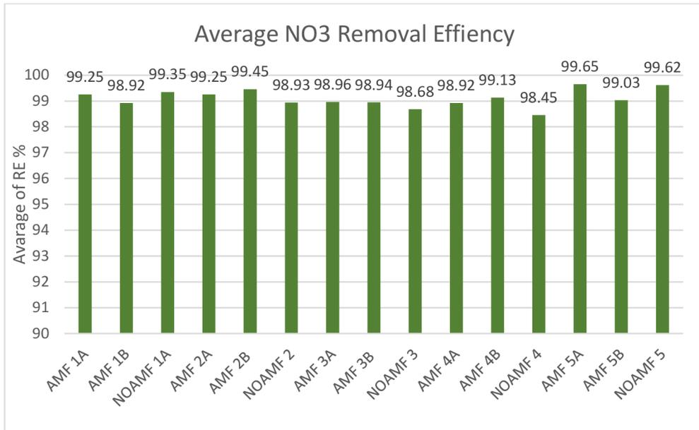
Figure 5.2.8 Average of Nitrates Removal Efficiency
