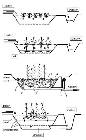
Figure  $N^{\circ}3.2.2$  -From Top to bottom - CW with free-floating plants (FFP), CW with free water surface and emergent macrophytes (FWS), CW with the horizontal sub-surface flow (HSSF, HF), CW with the vertical sub-surface flow (VSSF, VF). (Vymazal, 2001)
