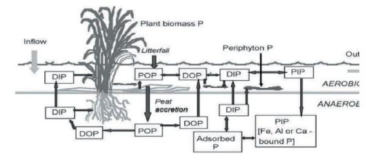
Figure N°3.5.3. Schematic showing phosphorus (P) cycle in wetlands. DIP = dissolved inorganic P; DOP = dissolved organic P; PIP = particulate inorganic P; POP = particulate organic P (Reddy and Delaune, 2005)
