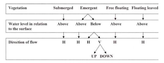
Figure  $N^{\circ}3.2.1$  The major characteristics of various types of constructed wetlands for wastewater treatment. H horizontal, V = vertical. (Vyzmal, 2010)
