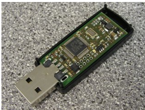
Figure 2.1: Entropykey: a hardware random number generator USB device. [13]
