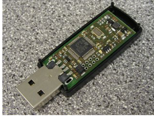
Figure 2.1: Entropykey: a hardware random number generator USB device. [13]
