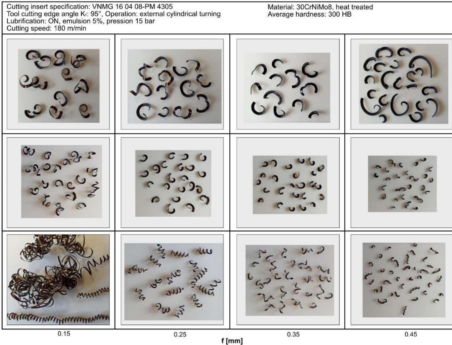
Figure 3.5.2.4 Chip fragmentation for semi-finishing with Sandvik indexable cutting insert VNMG 16 04 08-PM 4305.
