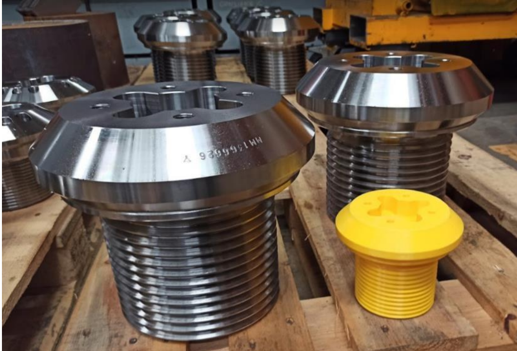
Figure 11 3D printed locking bolt HP6 (50% dimensions) next to the real size locking bolt HP6.
