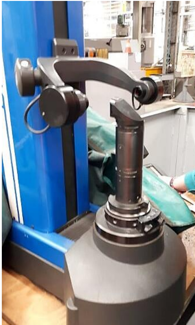
Figure 3.4.1.3 Roughing tool pre-setting using Trimos Optima tool pre-setter.
