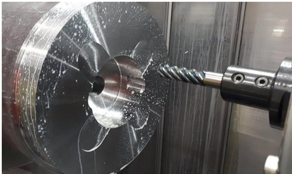
Figure 3.8.2.5 Safety test with offset in Z axis, depth of 1mm machined only.
