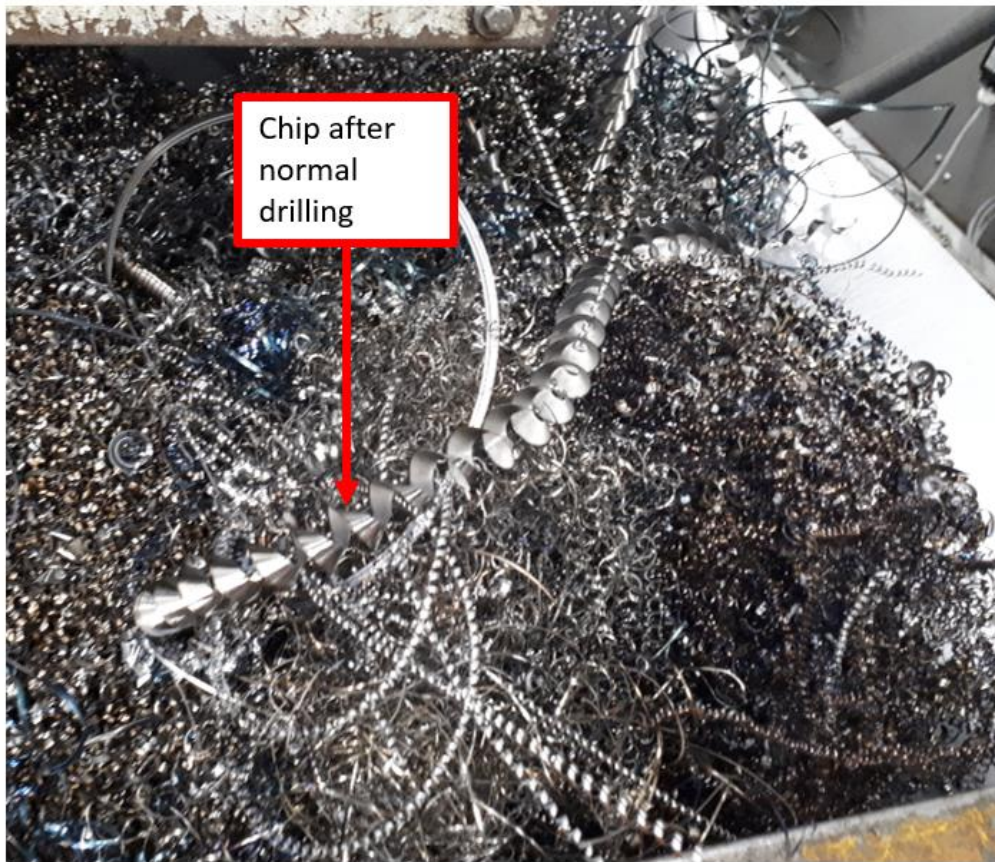
Figure 3.9.2.1 Chips after normal drilling (without chick peck cycle).
