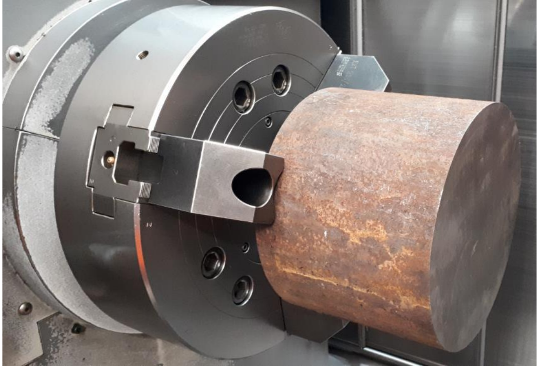
Figure 2.2.4.3 Workpiece with oxidized crust
