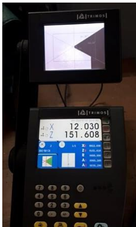
Figure 3.6.4.2 Tool pre-setter display while measuring of solid thread milling tool.
