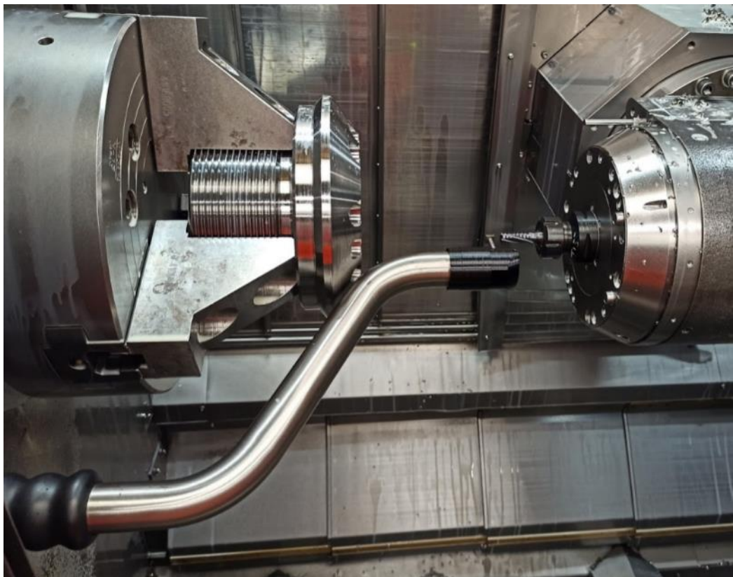
Figure 3.1.3.2 Renishaw HRPA tool setting arm in use during machining of a locking bolt.
