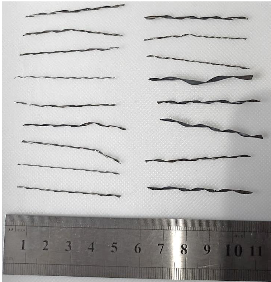
Figure 3.8.2.8 Chips from trochoidal pocket milling of 42 mm depth.
