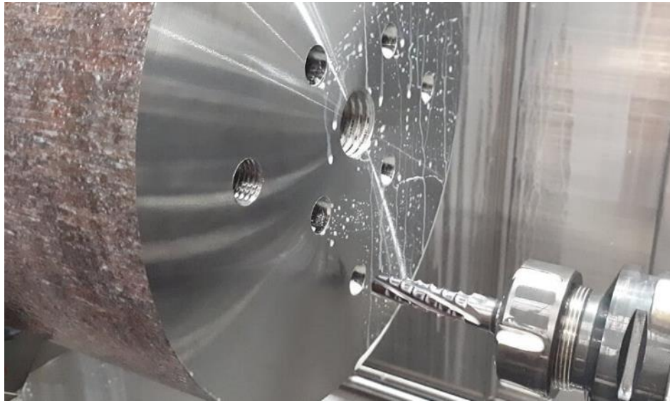
Figure 3.6.5.10 Workpiece and thread milling solid tool before machining of a thread.
