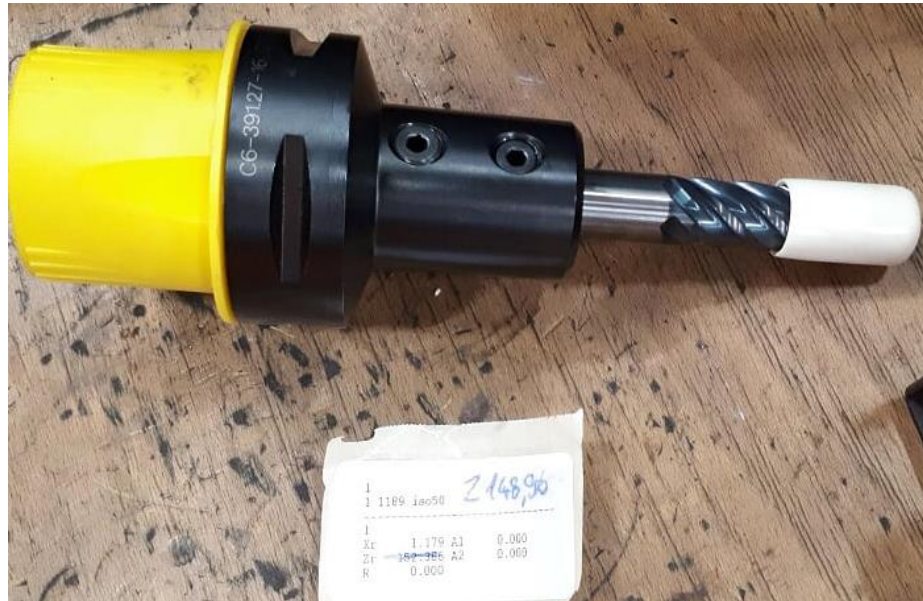
Figure 3.8.2.4 Milling tool MC122-16.0W5L-WJ30TF in toolholder and measured length and diameter by a tool-presetter.
