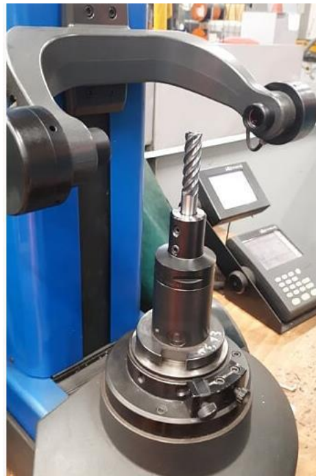
Figure 3.8.2.3 Tool set up using Trimos Optima tool pre-setter.
