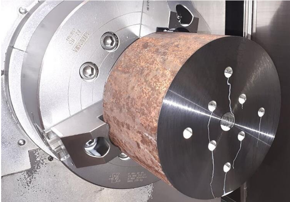
Figure -1 Workpiece for thread milling experiment prepared, face turned, drilled holes.
