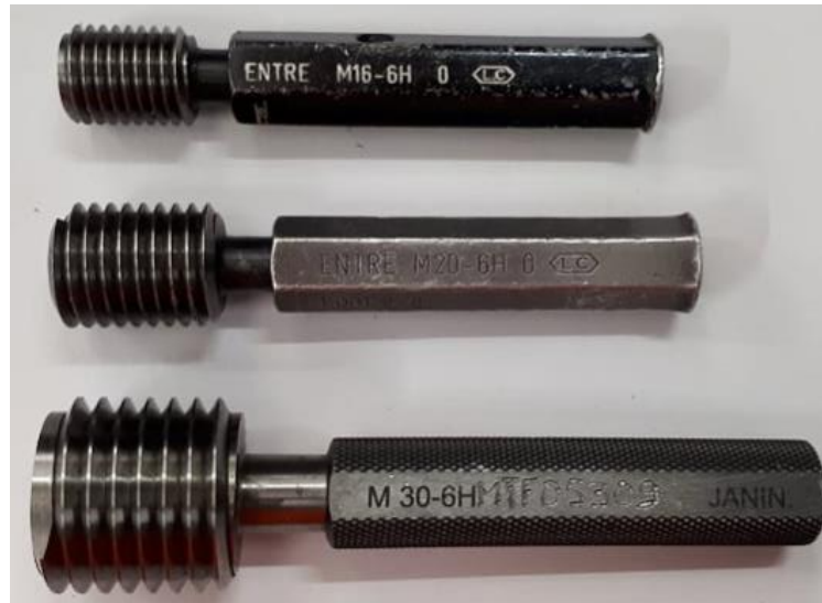
Figure 3.6.4.3 Thread gauges used for machined thread verification.
