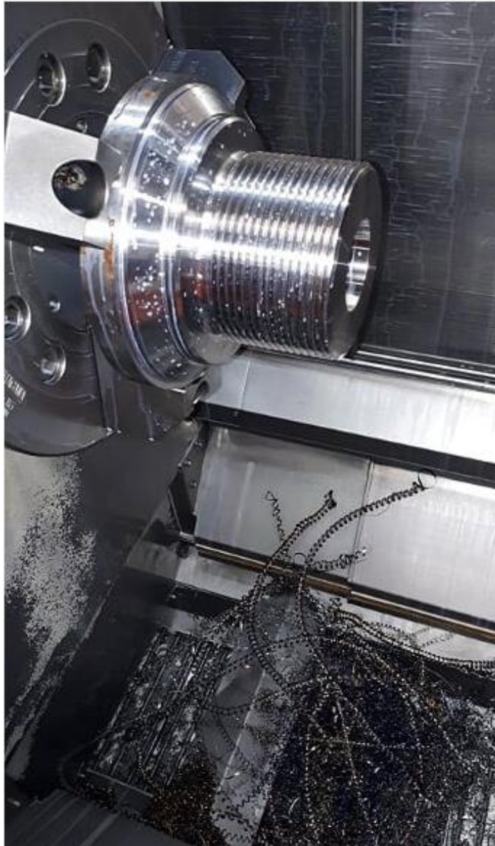
Figure 3.7.2.3 Workpiece and chips in chip conveyor after external thread turning with flank infeed.
