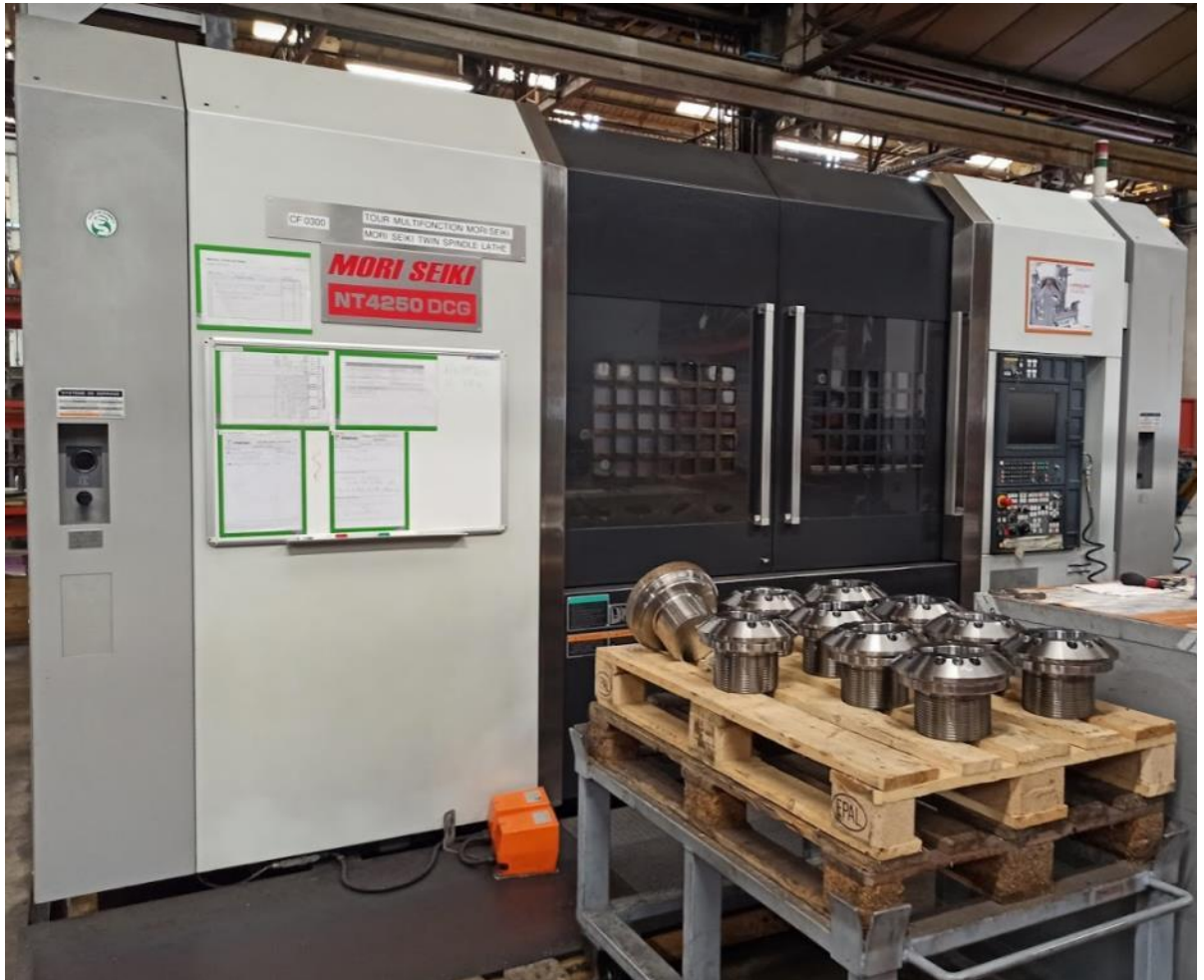
Figure 2.3.2 NT 4250 DCG Turn & Mill machine at Metso workshop with smaller locking bolts. Interior of the machine with chucks attached to both spindles is displayed in the figure below.
