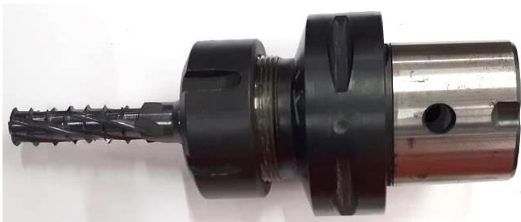
Figure 3.6.5.9 Tool TC620-M16-A1E-WB10TJ in toolholder.
