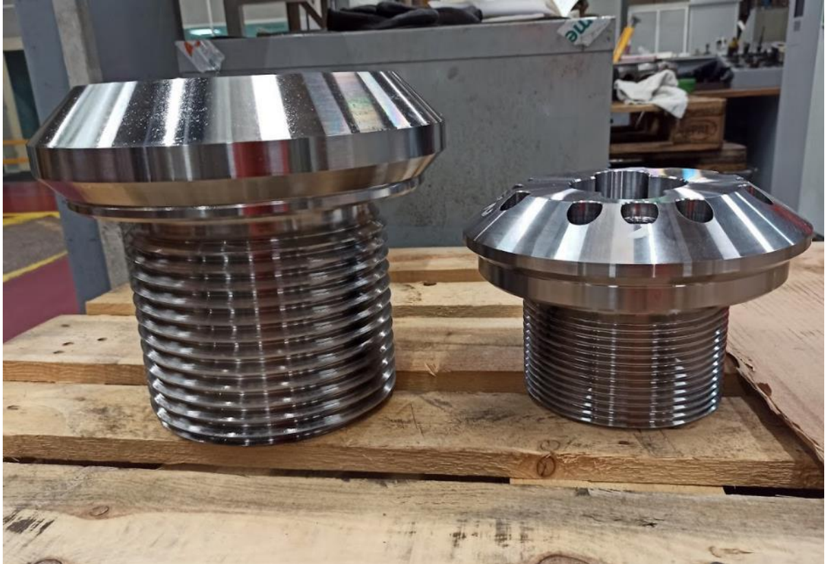
Figure 2.2.1.4 Difference of scale between two head bolts: HP6 (left) and HP200 (right).
