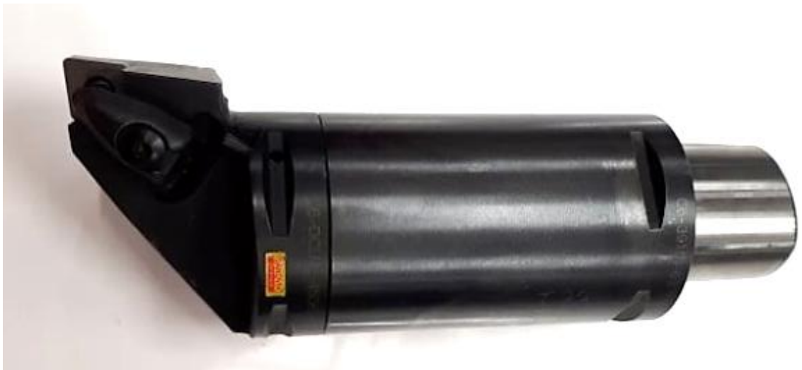
Figure 3.4.1.2 Toolholder C6-DCLNL-45065-16 with attachment C6-391.01-63 100A.
