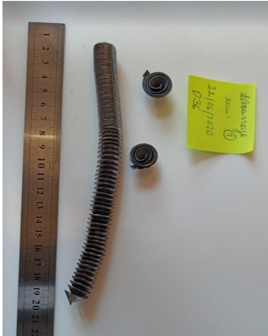
Figure 3.9.2.2 Chips obtained using chip peck cycle during drilling G3 (all three chips are from the same cycle).
