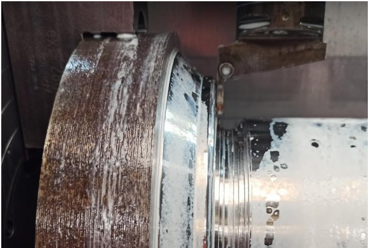
Figure 3.9.1.1 Grooving insert and roughing of the groove.
