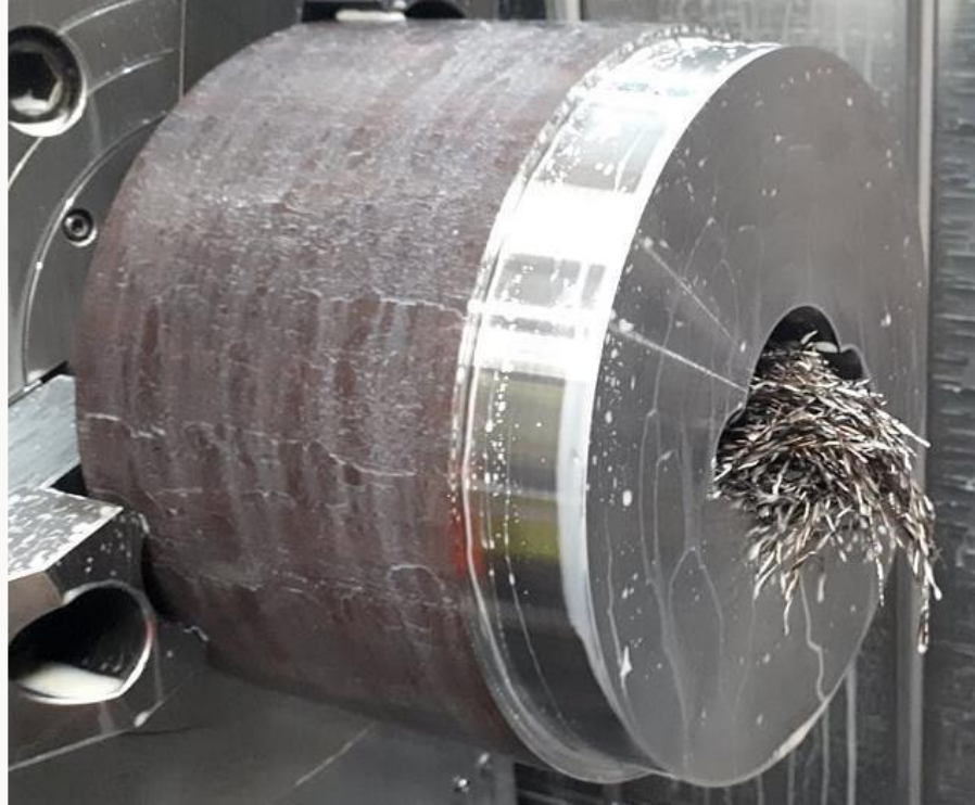
Figure 3.8.2.6 Pocket after trochoidal milling, illustration of chip evacuation problem.
