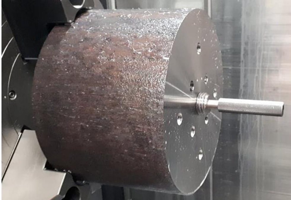
Figure 3.6.5.5 Thread gauge inserted in the machined threaded hole.
