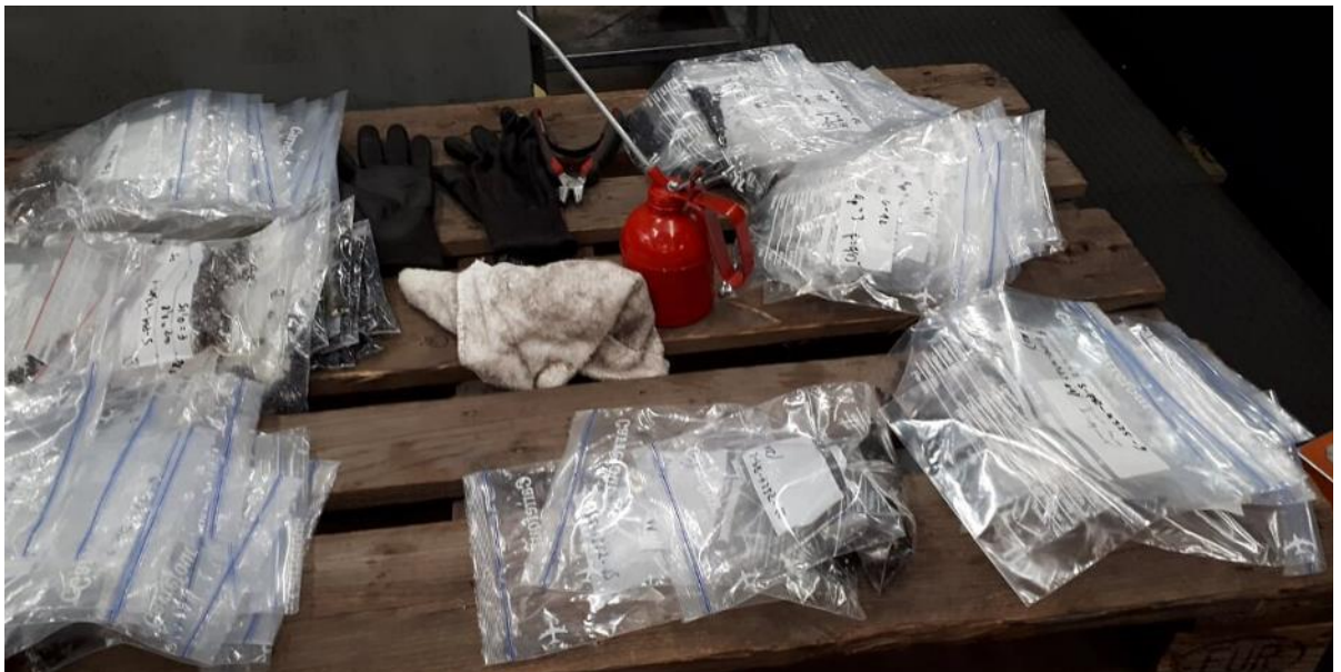
Figure 3.4.3.4 Chip samples in labelled zip lock bags after adding oil to protect chips from corrosion.
