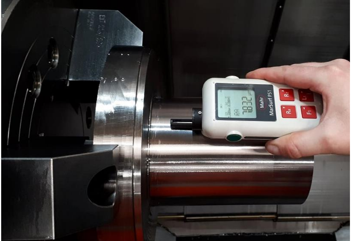
Figure 3.5.3.2 Measurement of surface roughness with a roughness tester.
