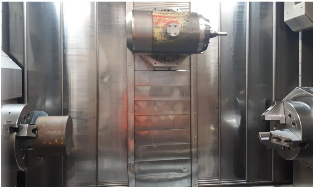
Figure 2.4.1.1 Workpiece clamped for operation 1.
