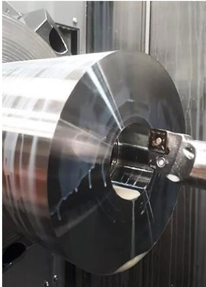
Figure 3.6.2.2 Workpiece and tool during experimentation of boring.
