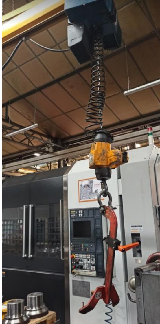
Figure 2.2.4.5 Manipulation jig attached to a crane.
