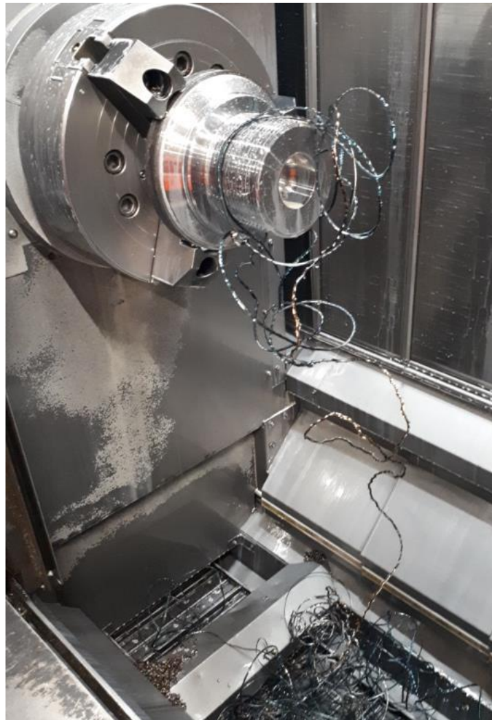
Figure 3.7.2.2 Chips after machining the external thread with radial penetration mode for locking bolt HP3 (M140x6) in original cutting sequence.
