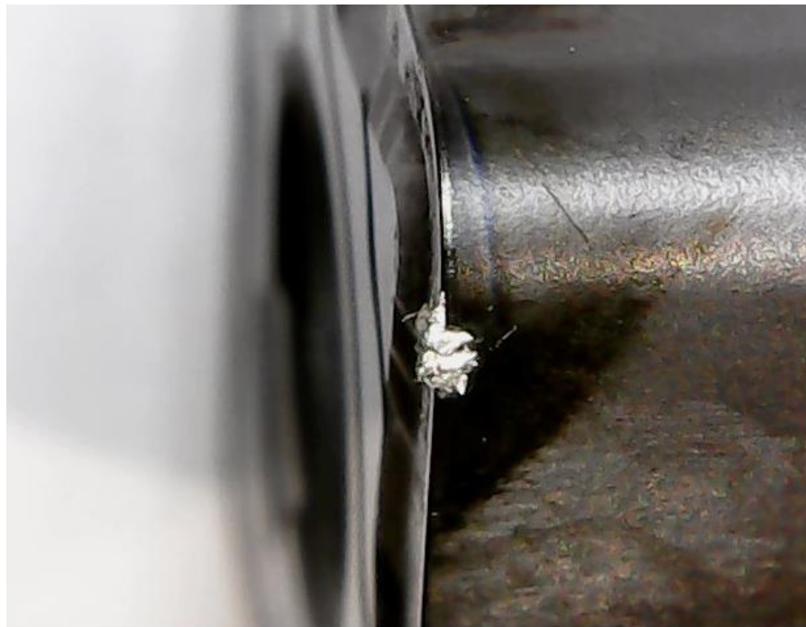
Figure 3.4.6.2 Groove shape wear typically obtained after roughing operation of the locking bolt.
