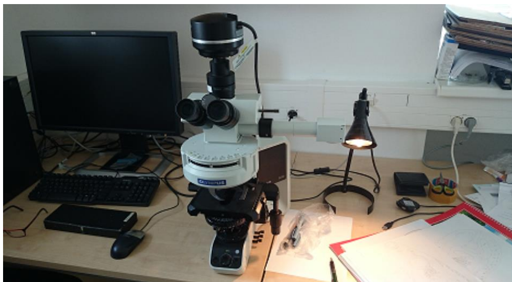
Fig. 19: Drawing and measurement with BX53 with optical device DP 72 and camera lucida .
