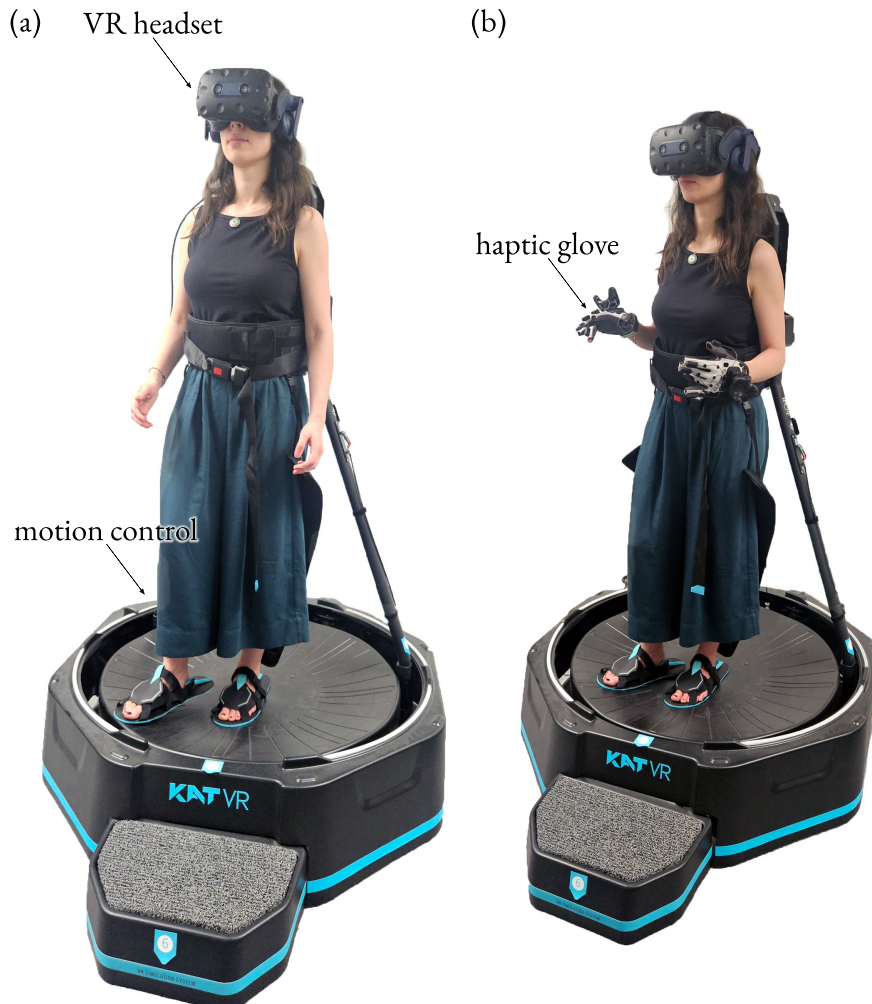
Figure 27: Participant using VR headset in a room, standing in a motion control station, (a) bare handed and (b) wearing haptic feedback device
