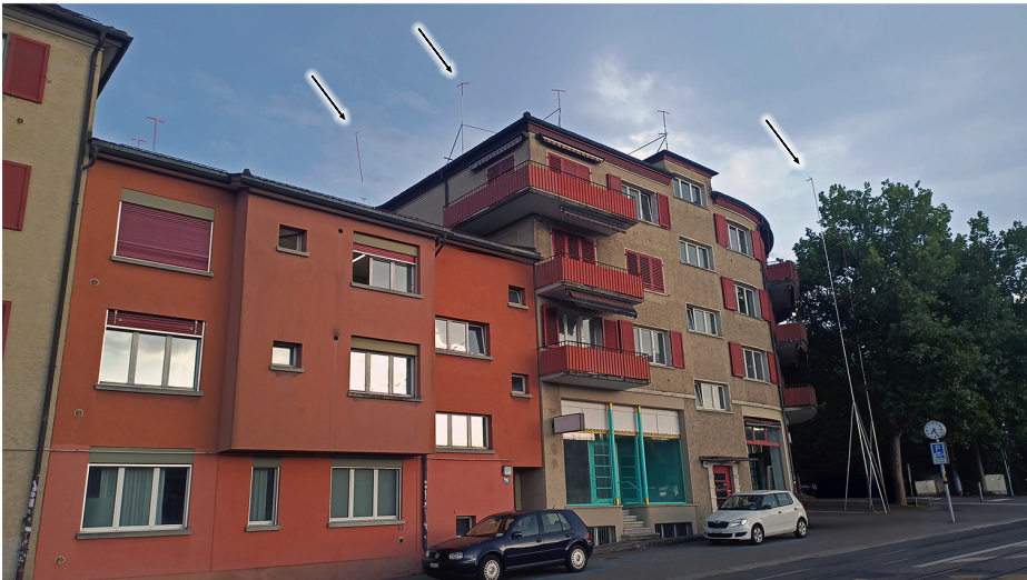
Figure 10: Baugespann from the participants' perspective; three arrows point to the top of the poles determining the volume of future development
