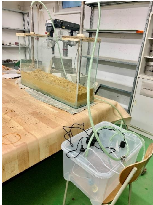
Figure (7) is the prepared cubed EOR model in the lab which it has two wells (injection and production), water tank and sand reservoir layer.
