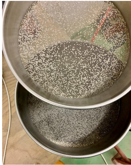
Figure (18) is showing both sieves which used for sand grains. The upper one is (1) mm and the lower one is (0.5) mm.
