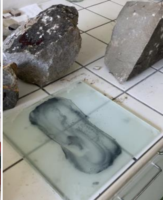
Figure (b) is fine abrasive with water are applied to glass bride.
