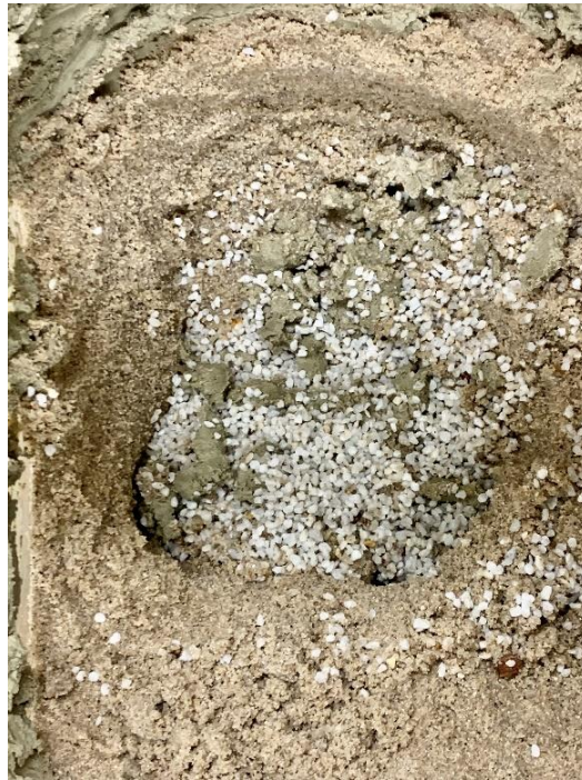
Figure (23) is the added clay around the perforated zone of the production well to damage it and decrease the permeability. Then, monitored that, if it can be improved by electrical currents.
