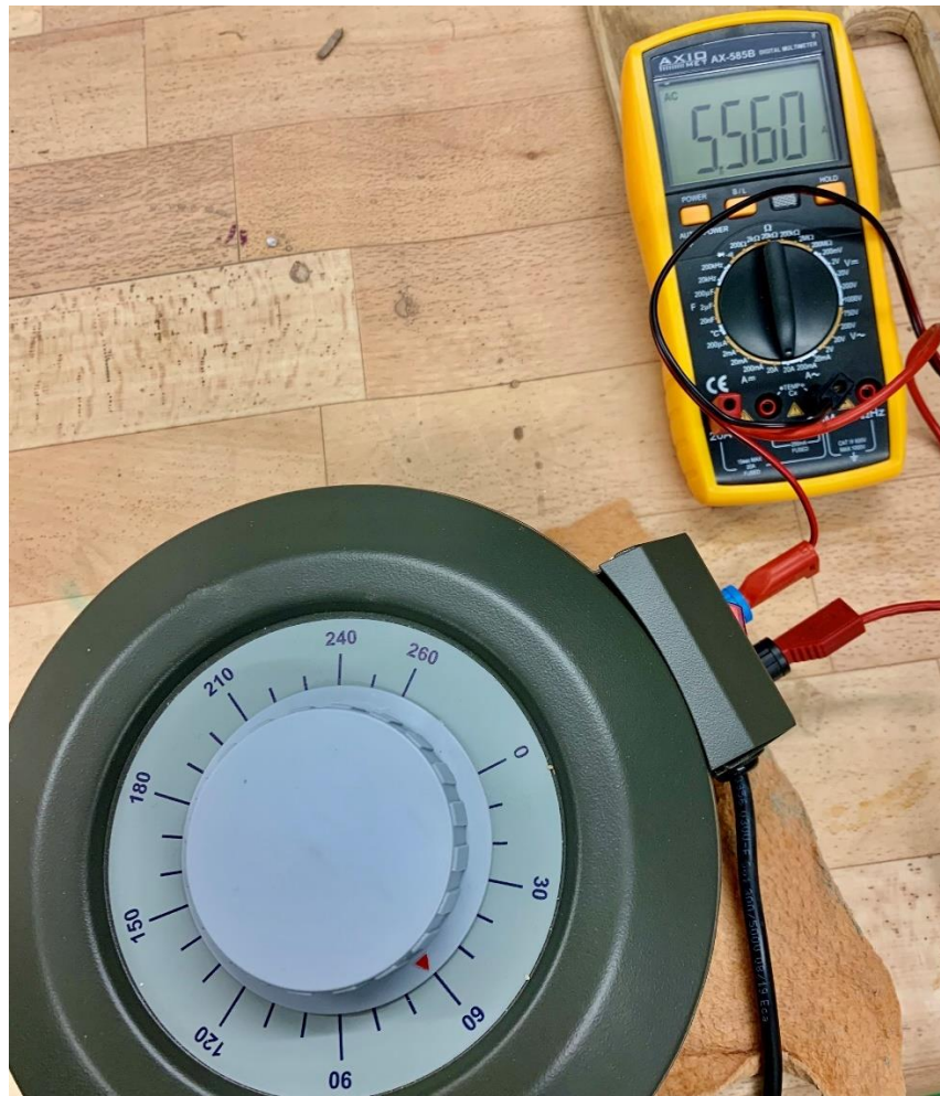
Figure (35) is showing Both of auto transmitter with the multimeter. Approximately (60) V is applied to the model during the electrostimulation. For the force of (60) V, (5.5) A of electrical current are generated. For (20) min the electrostimulation is continued by that value.
