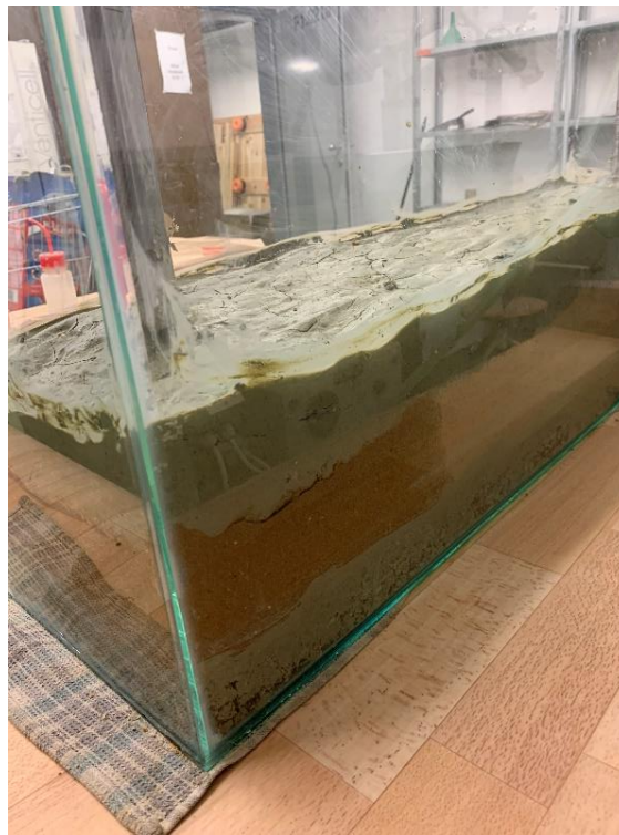
Figure (28) is showing the front during water saturation of the permeable sand layer, in the first test. The water is injected from the injection well to the production well.
