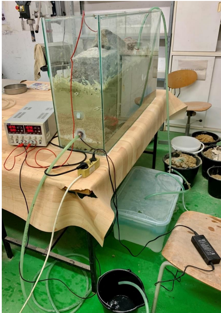
Figure (33) is showing the electrostimulation by using the DC current. The circulation is started as a stable manner. The power supply relates to the EOR lab model by two wires. The wires are interlinked with the electrodes (injection and production wells) separately.
