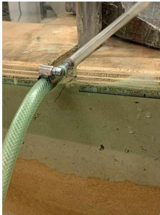
Figure (13) is showing the drilled glass and interlinking the hose from the head of the shortened production well to the water tank in the lower height level.
