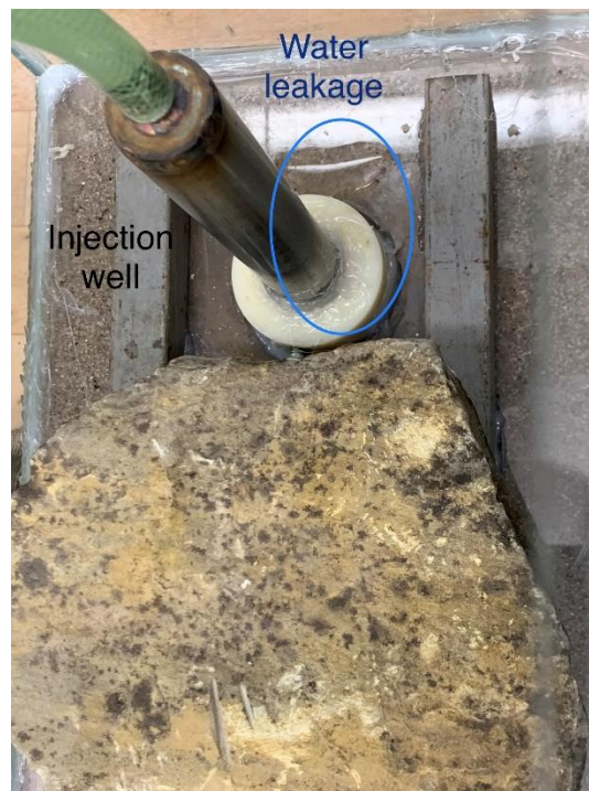
Figure (45) the water leaking through the spaces between the injection well and the polycarbonate which blocked by silicone, but it is opened by salt water with high pressure.
