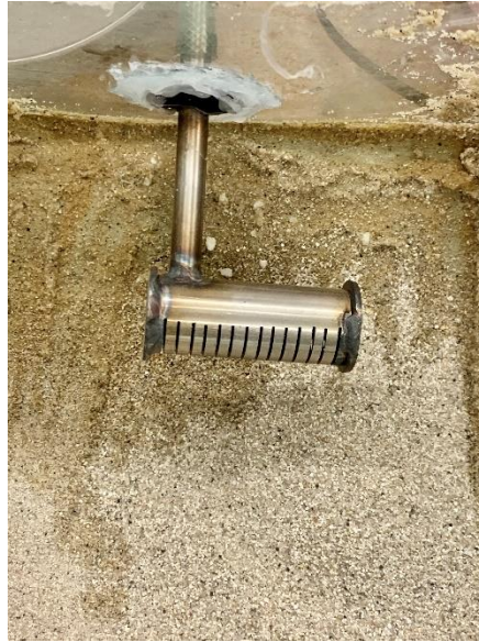
Figure (19) is new production well which is applied to the model horizontally inside the permeable sand grains, with new a shape of the perforation holes.
