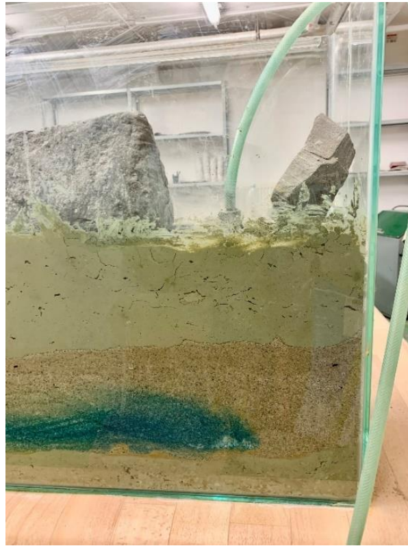
Figure (48) is presenting that, the blue ink is injected to the EOR model through the injection well. Coarse gravels around the injection well are fulfilled with the ink then the ink swept water towards the production well through high permeable zones.
