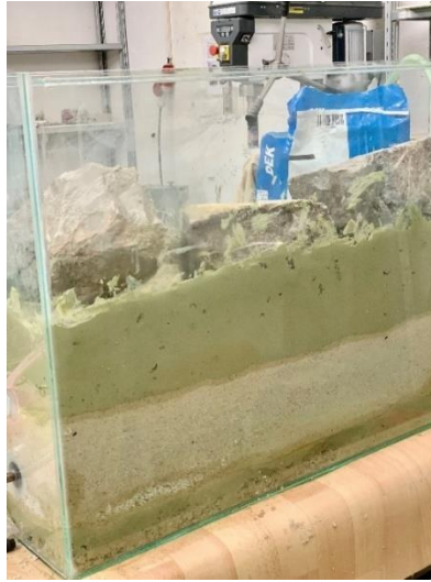
Figure (20) the new design of the model can be seen by increasing thicknesses of both of sand layer and sealed clay layer. Coarse gravels can be seen near production well by white color inside the permeable sand layer.
