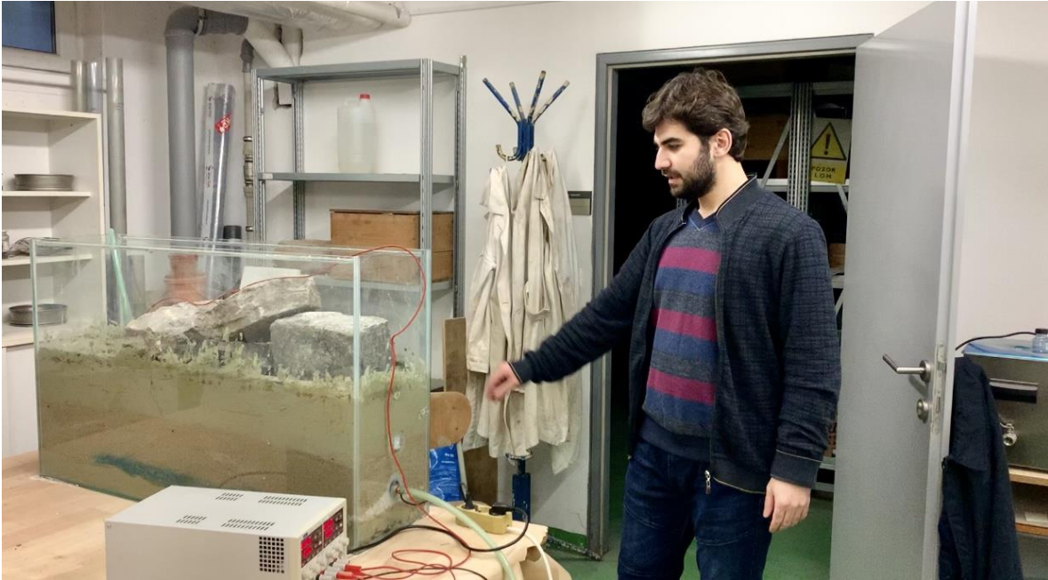
Figure (25) is showing the DC power supply which applied to the model by interlinking electrodes with the power source by two wires.
