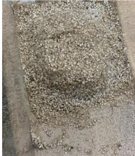
Figure (14) is showing that coarse gravels are placed around both injection and the production wells in the perforation zone.
