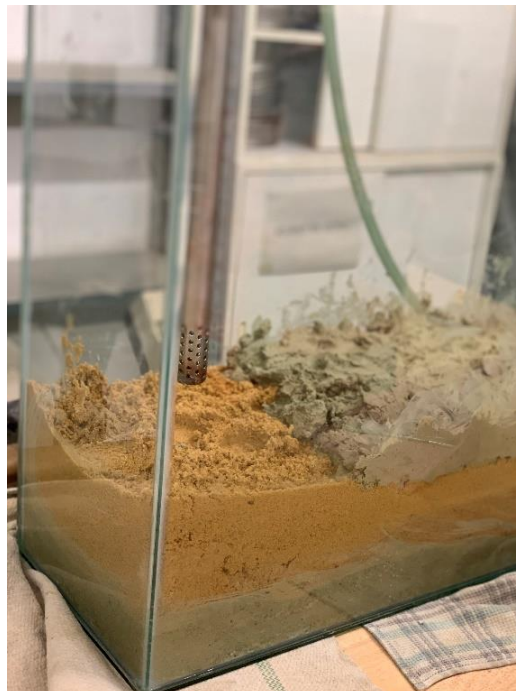
Figure (8) is showing that the production well is perforated and dropping it to be applied onto the sand medium grains as a reservoir layer. From the figure, the sand layer has yellow color.
