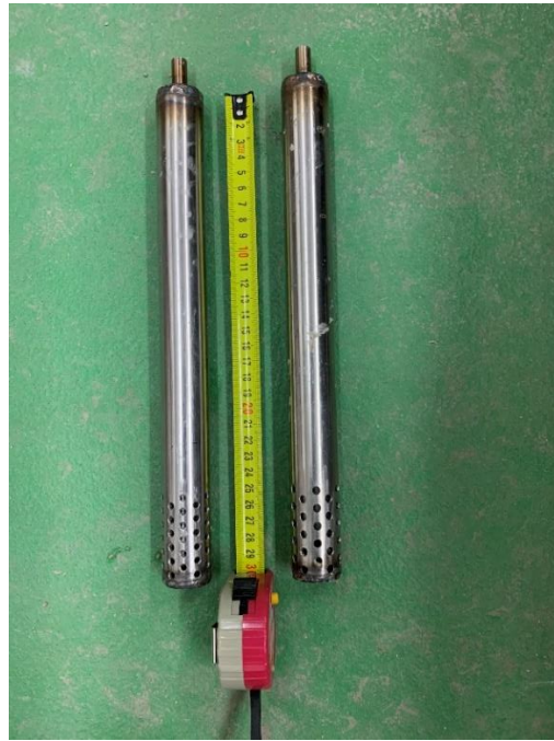
Figure (12) is showing both of shortened production and injection wells which the length of them reduced from (100) cm to (30) cm.
