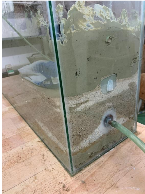
Figure (46) the last design of the EOR lab model which the sand reservoir layer is saturated with water from the injection to the production well. The hose as can be seen is connected with the production well. The water produces and goes to the water tank.
