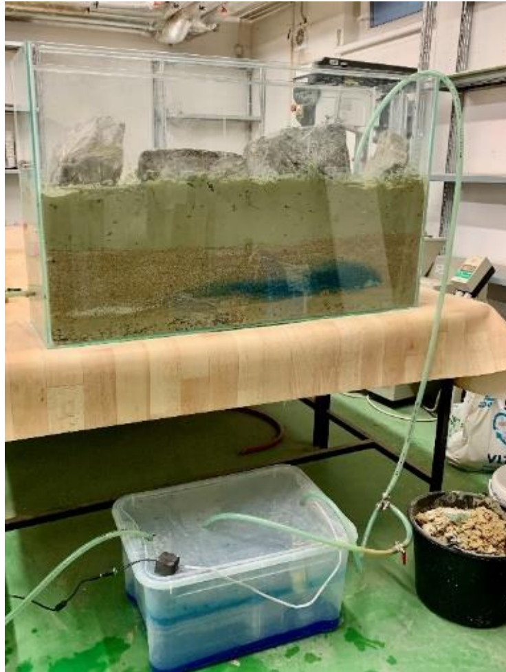
Figure (32) is showing the ink injection as a tracer. The ink is showing the highest permeable zone from the sand reservoir layer, by blue color.
