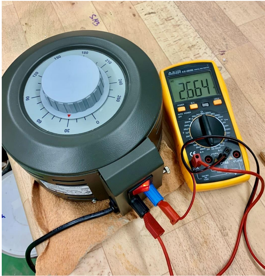
Figure (34) is showing Both of auto transmitter with the multimeter. Approximately (30) V is applied to the model during the electrostimulation. For the force of (30) V, (2.6) A of electrical current are generated. For (20) min the electrostimulation is continued by that value.
