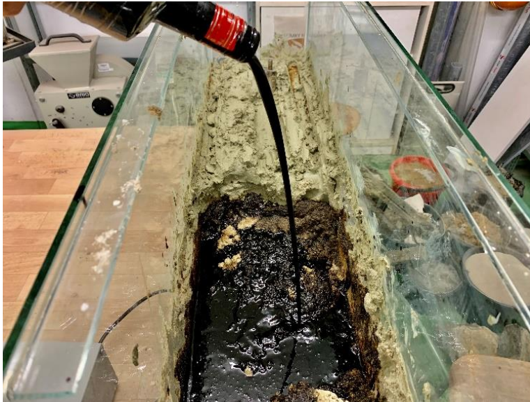
Figure (26) is presenting that the sand layer inside the EOR lab model, is saturated with the heavy crude oil. Then, sealed clay layer is placed above.
