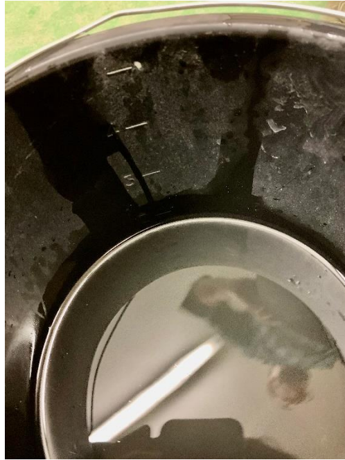
Figure (47) the bucket which the produced flow rate is measured manually. The hose which connected the production well with the water tank, took out from the water tank and put into the bucket, time is set-up, the flow rate was (2) L/min.
