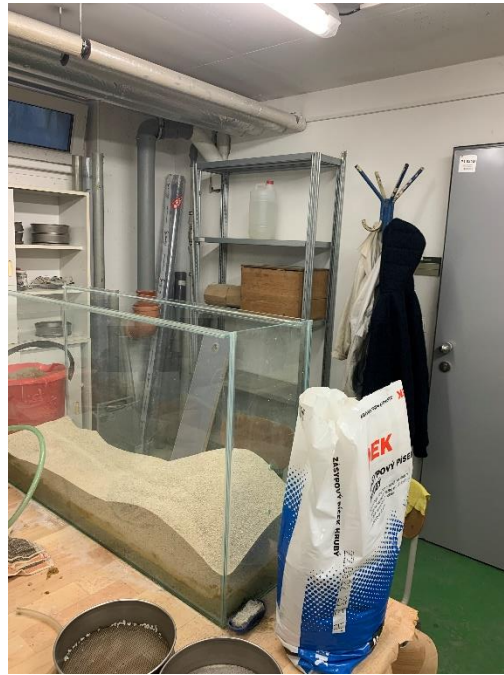
Figure (16) is showing the reservoir cubed model which the sand layer is changed to the new sand layer which grain sizes were between (0-1) mm.
