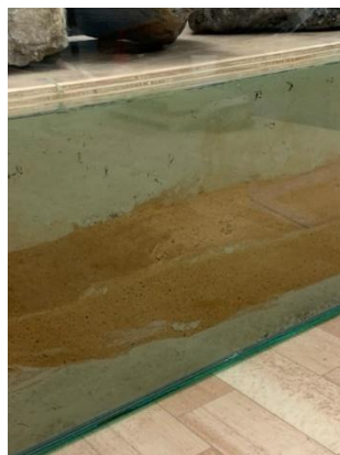
Figure (10) is showing preparation for the second test of the model before the Electrostimulation in order to get successful circulation. The thickness of the sealed clay layer is increased, and the compacted wooden layer is placed above with rock samples.
