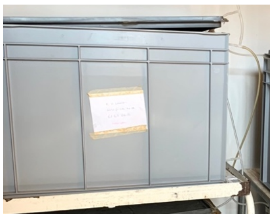
Figure 8: Set up of incubation of fertilizer for the hydroponic growing experiment. The bin contains 50 L of double-distilled water mixed with soil-inoculated organic fertilizer mixed.
