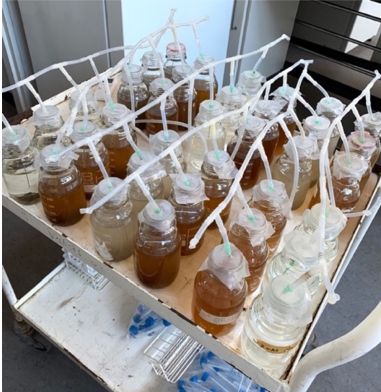
Figure 7: Set up of incubation experiment. Aeration setup and bottle placement are visible. The temperature and humidity meter is seen on the left side of Figure 7b.
