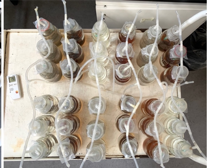
Figure 7: Set up of incubation experiment. Aeration setup and bottle placement are visible. The temperature and humidity meter is seen on the left side of Figure 7b.
