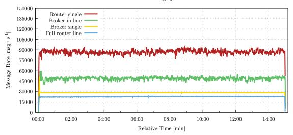
Figure 6.8: The comparison of all measured throughputs for different components and topologies.
