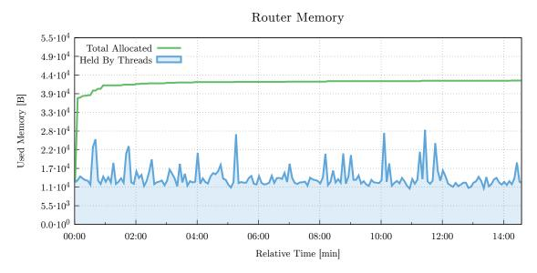
Figure 6.3: The total allocated memory and memory-in-use by message router during the test. The data was collected by the inspector every 5 seconds.
