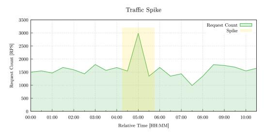
Figure 2.2: The graph shows amount of concurrent sessions depending on time. During to network traffic monitoring we can see the traffic spike occurring after five hours from test start.
