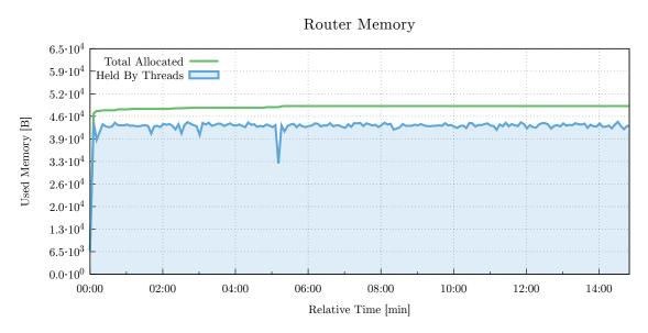
Figure 6.6: Message router's memory usage during the multipoint case study. Used memory is higher than in the single-point.
