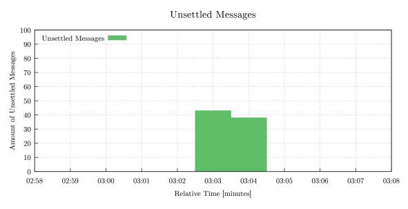
Figure 6.22: Chart captures unsettled messages on the redundant router node. The slave router handled load for two seconds.
