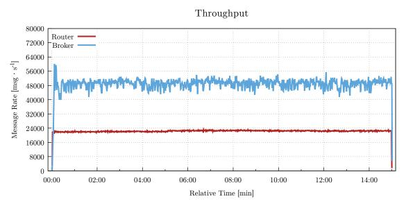
Figure 6.5: Measured throughput of message router and message broker during the multipoint case study. One can see the performance degradation of message router and improvements of message broker on that Figure.
