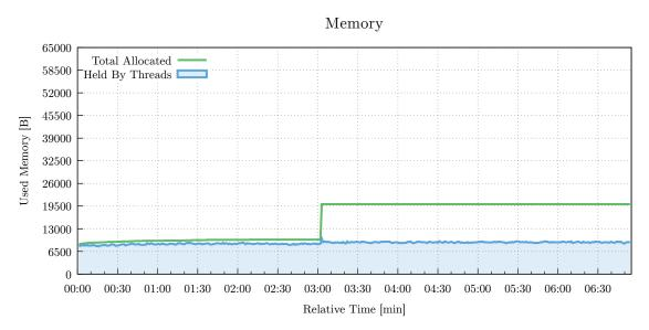
Figure 6.20: Allocated memory for redundant router during the restart. One can see that router allocated new memory when the master router crashed and the slave had to handle the load. This memory is allocated until the tear down.
