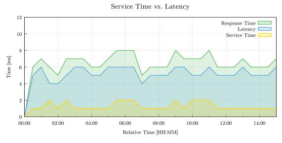
Figure 2.7: Diagram capturing the difference between the latency and response time.
