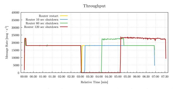
Figure 6.17: Maestro Agent demonstration against a simple topology with restart and shutdown in the third minute of test.
