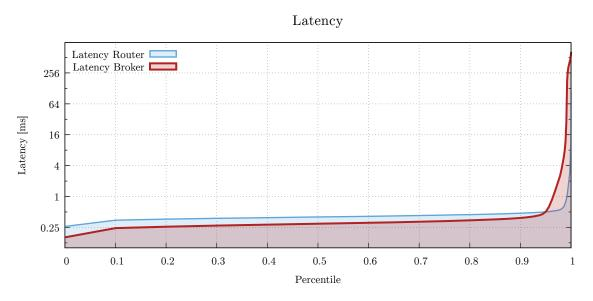
Figure 6.10: Latency chart showing the difference between the router and the broker latency at same load. Router's latency is significantly better then in previous case.
