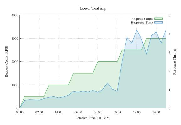
Figure 2.3: The response time of the system during the load testing depended on requests per second.
