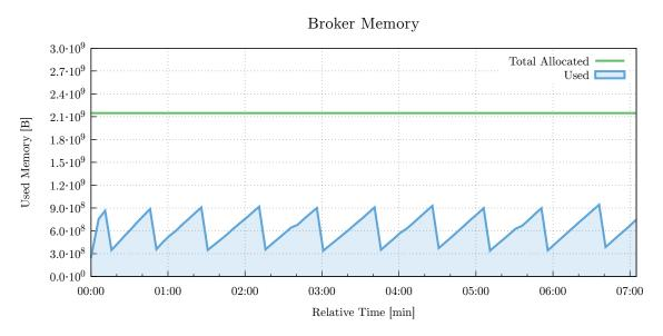
Figure 6.12: The Broker's memory usage has less spikes when the load is only about of 80% of maximum.
