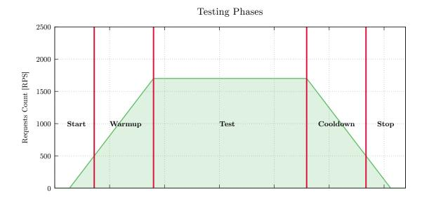
Figure 2.6: Load phases of performance measurement process.
