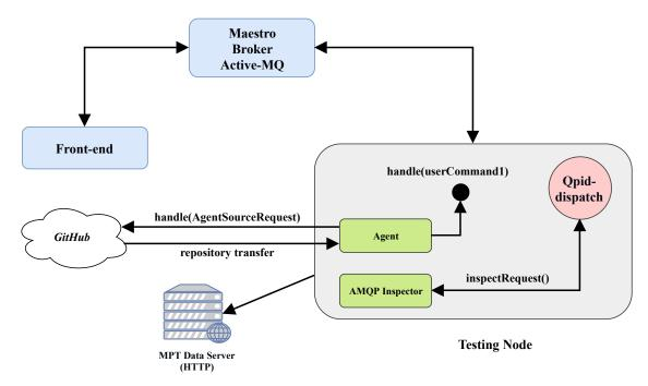
Figure 5.1: Communication scheme inside the Maestro with the agent. Scheme shows the agent git repository download and then handling the proper note defined by the user. The Figure also shown the SUT communication with the AMQP Inspector.
