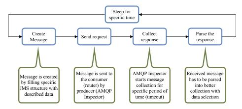
Figure 5.3: The whole Inspector process including message creation, message sending, collecting and parse.
