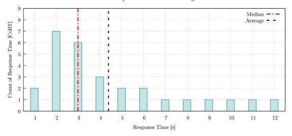
Figure 2.8: Transactions response time with calculated average and median of response time. The average represent inaccurate response time, which is higher than real one.
