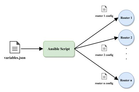
Figure 4.4: The scheme of configuration files deployment to the nodes The Ansible script takes input file with variables generated by Topology Generator, fills the configurations template and deploy them to corresponding nodes.
