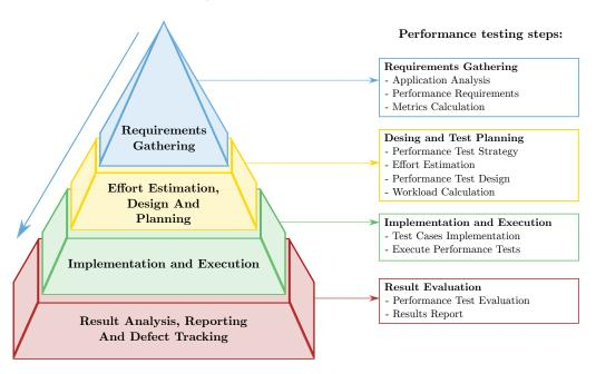
Figure 2.1: The performance testing process with the four most important parts and theirs individual steps based on [24].
