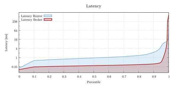
Figure 6.9: Latency chart showing the difference between the router and the broker latency at 80% of maximum rate.
