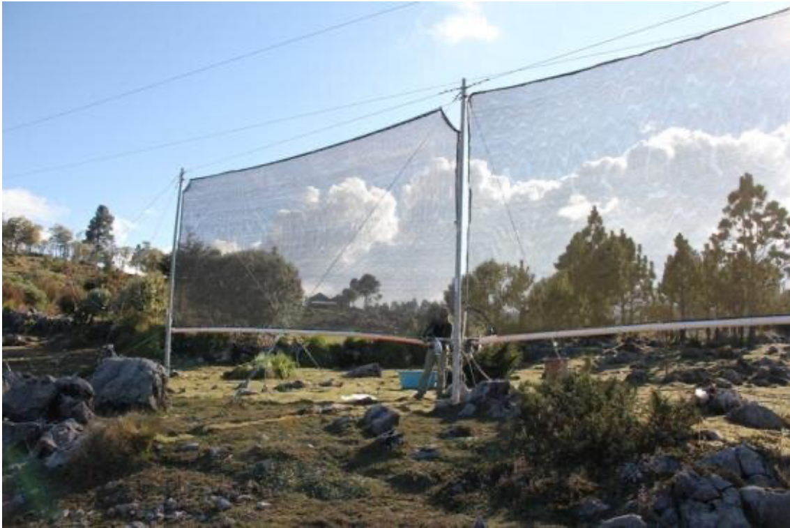
Figure 17 Two Large Fog Collectors in Tojquia (Schemenauer et al. 2016)
