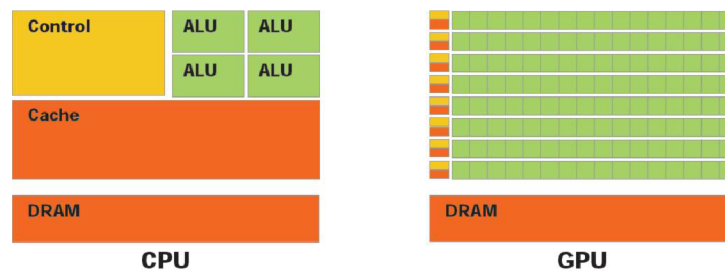
Figure 2.5: CPU and GPU Architecture Overview. [64]
