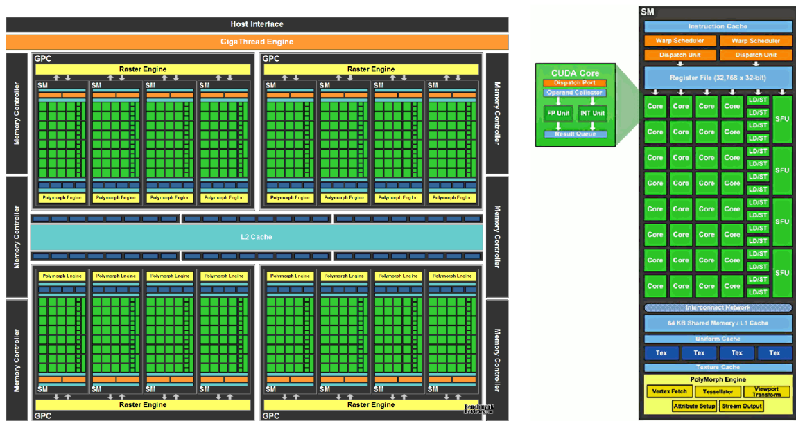
Figure 2.13: Fermi Architecture GeForce GT300 (GF100).
