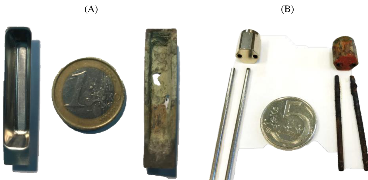
Figure 8 The corrosion and wear effects to TD-AAS during the direct analysis of fish sauce samples. Sample boat (A) and sample boat holder (B) before (left) and after (right) several runs of direct analysis.
