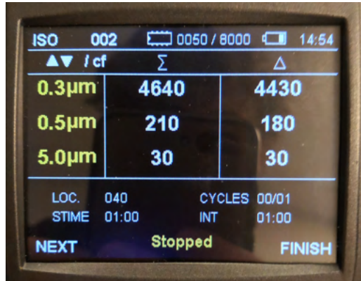
Figure 3.13: Results of the measurement of the number of particles in the room
